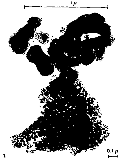
FIGURE 4. AGGREGATE STRUCTURE OF ALUMINA I PARTICLES
