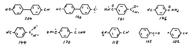
The major part of the sublimate condenses in the top part of the cell. The yellow product melts between 178 and 198°C. Its mass spectrographic analysis exhibited major peaks at 128 and 118 and minor ones at 101 and 91. The following assignments can be made:
