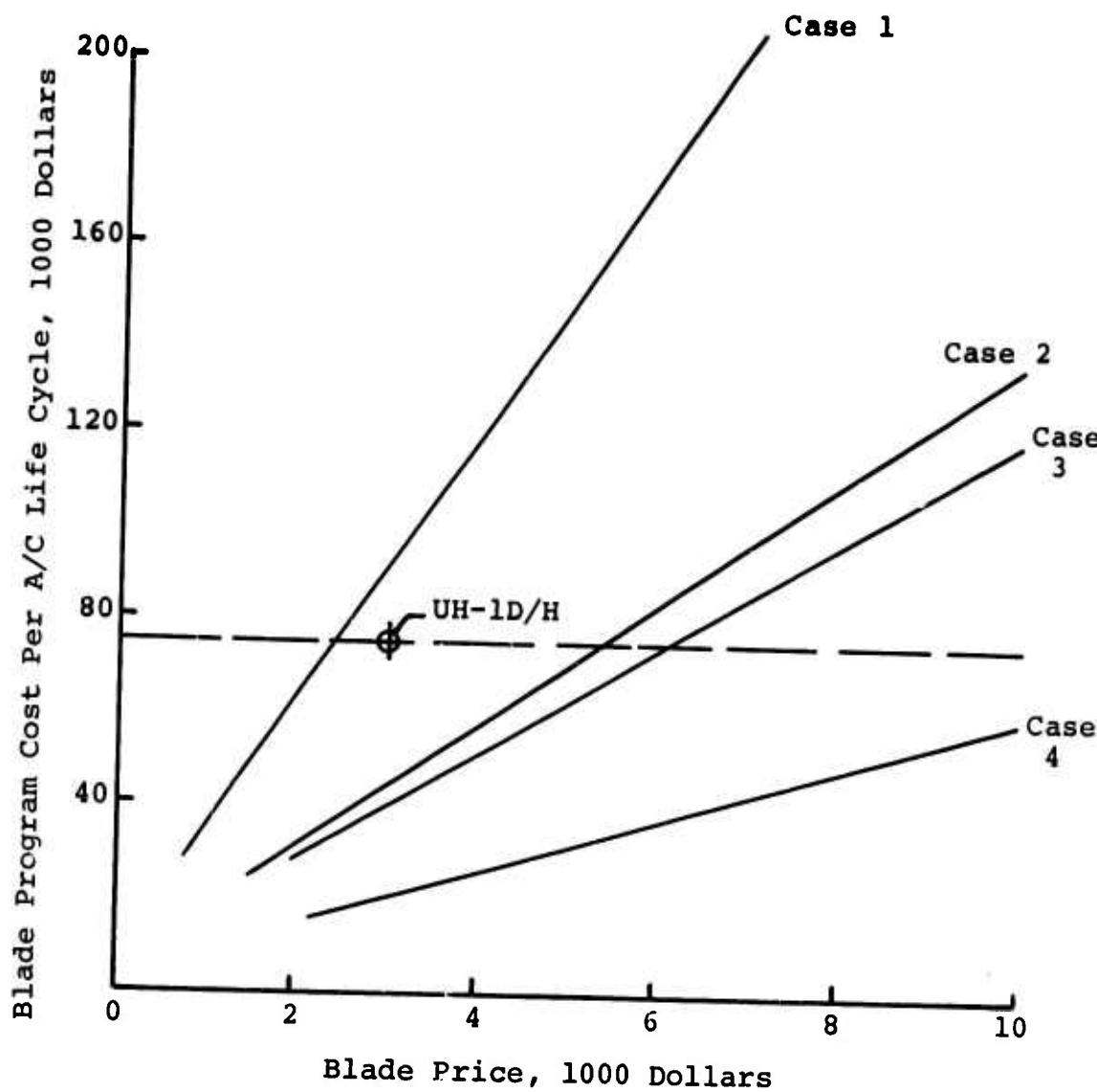
Case 1 - Nonrepairable, all damage scrapped
