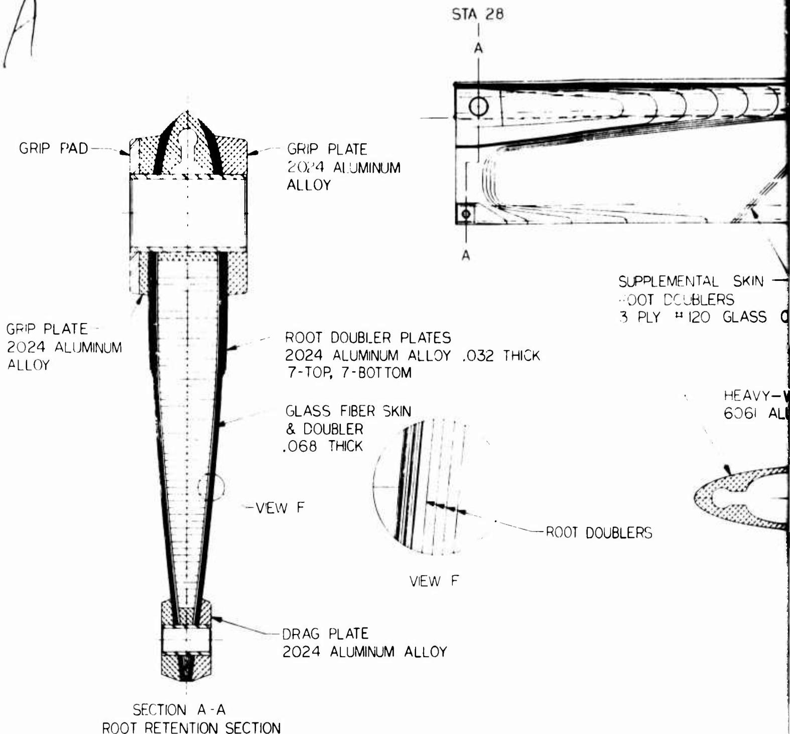
Figure 6. Configuration V, Selected Repairable Rotor Blade Design.
