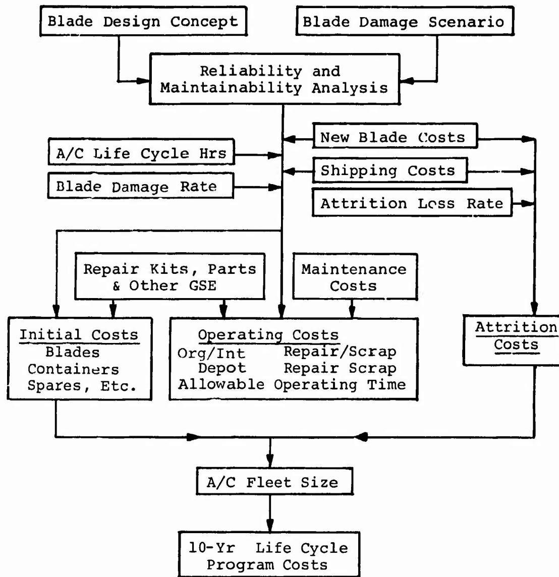
Figure 5. Cost Model, Rotor Blade Life-Cycle Costs.
