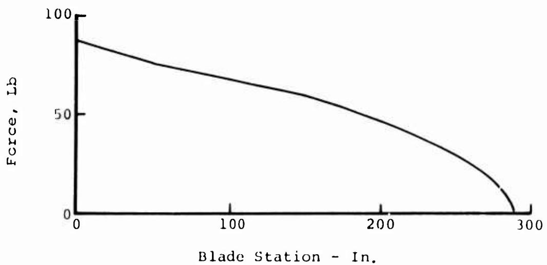
(a) Centrifugal Force at a Rotor Speed of 315 rpm for the UH-1H Blade.
