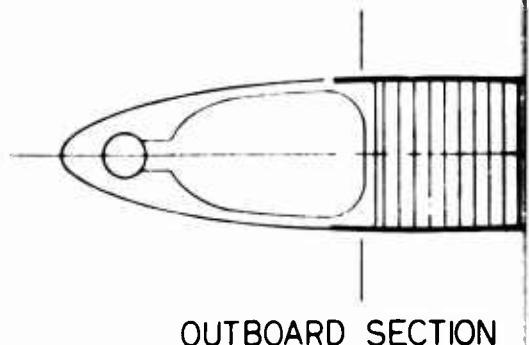
Figure 9. Configuration III, Repairable Rotor Blade Using Heavy Wall Aluminum Spar.
