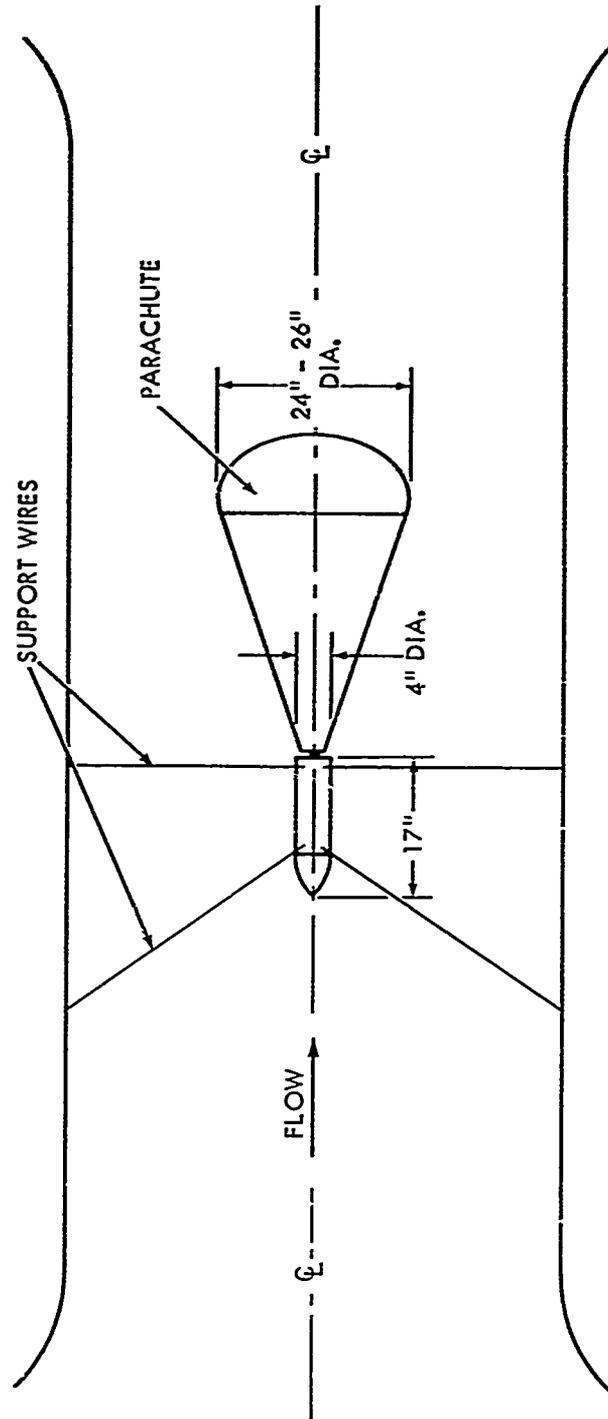
WIND TUNNEL CROSS SECTION DIMENSIONS 7 FT x 11 FT
