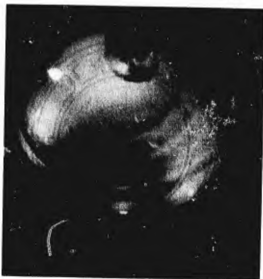
Fig. 14 Motion of Mode V. s = 12.15 mm, Re = 1,210 , Ta = 95.6
