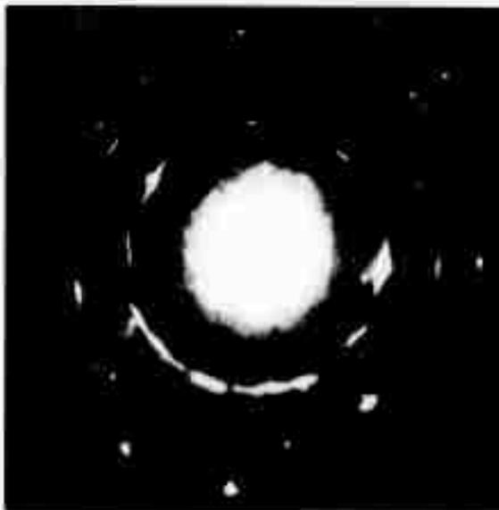
Figure 10. Electron Diffraction Kikuchi Pattern from  $(01\bar{1}2)$   $Al_2O_3$  (Neg. 1510)
