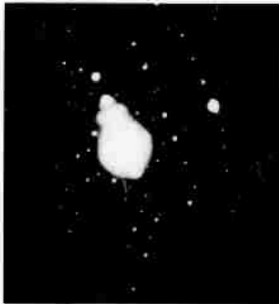
Figure 9. Electron Diffraction Spot Pattern from  $(01\bar{1}2)$   $Al_2C_3$  (Neg. 1506)
