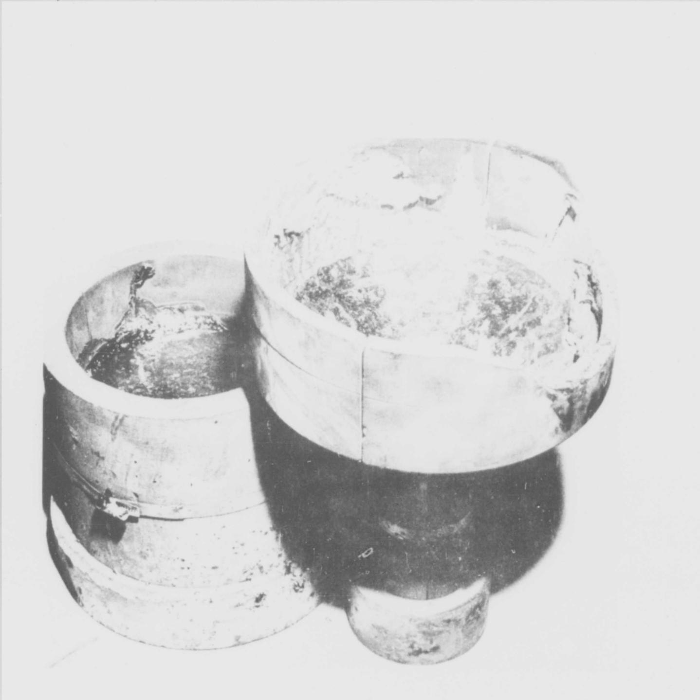
FIGURE 3. - Skull casting removed from mold
