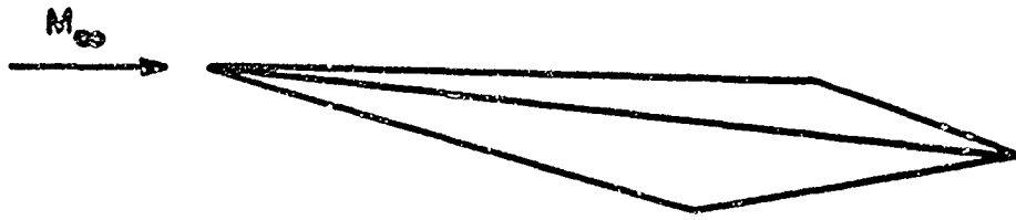
Fig.6 Optimum wing (Best L/D) according to Newtonian theory
