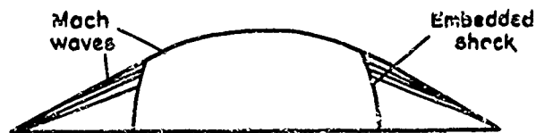
Fig.2 Flow past upper surface of a delta wing (after Babaev)
