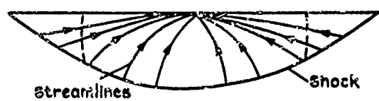
Fig.1 Flow past lower surface of a delta wing (after Babaev)
