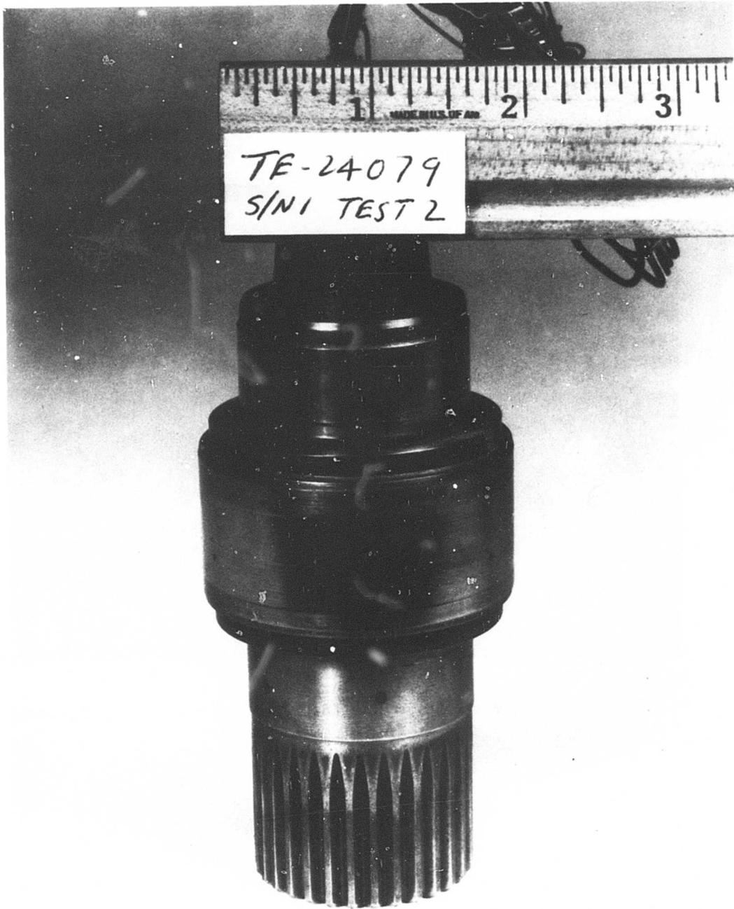
Figure 39. Inner Race Following Differential Speed Test, Design A.
