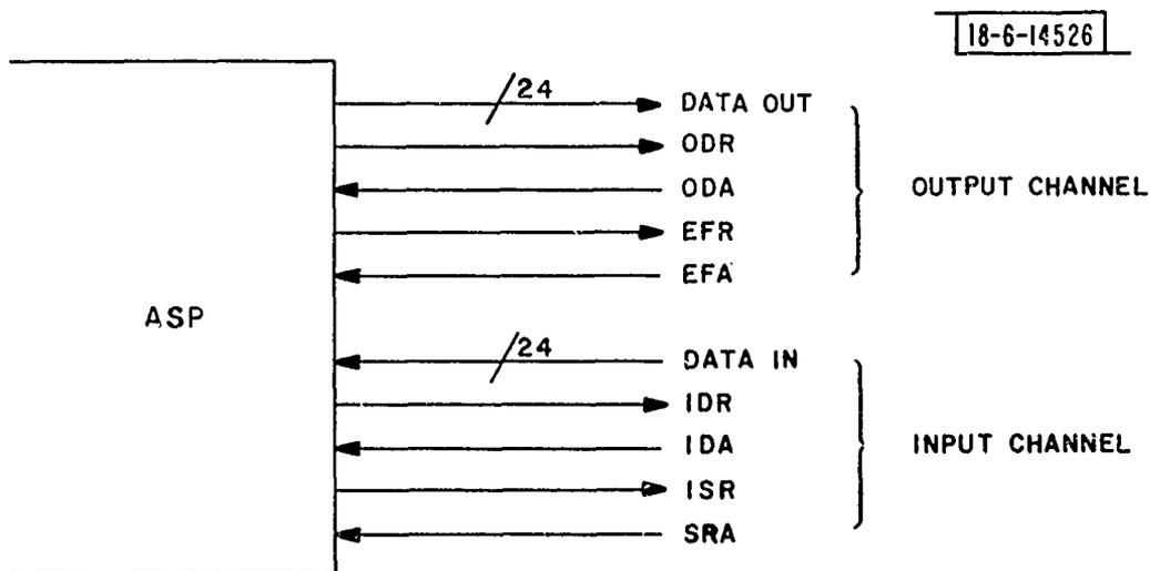
Fig. 30. Direct memory access channel.
