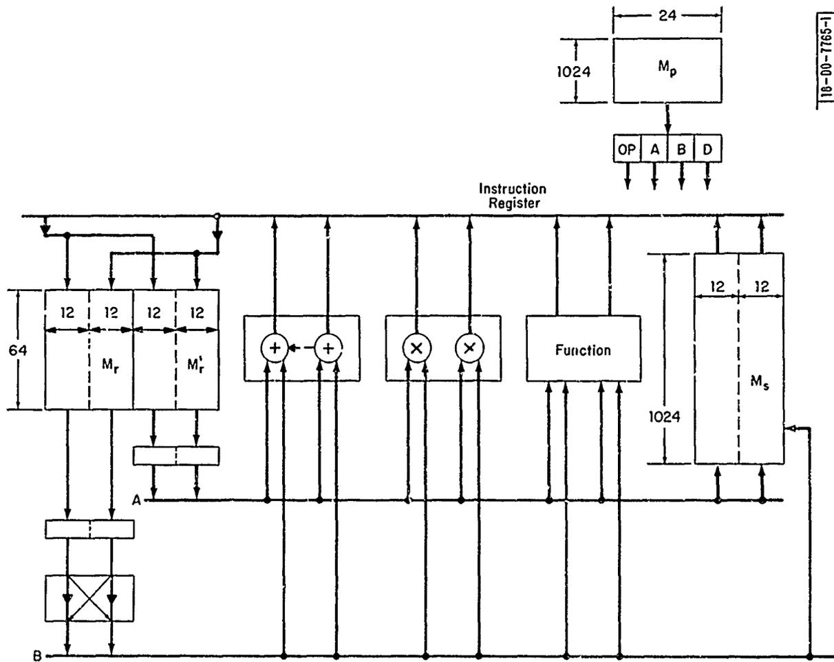
Fig. 3. Structure of the Advanced Signal Processor.
