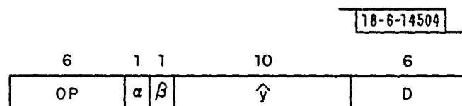
Fig. 5. Format for arithmetic jumps.
