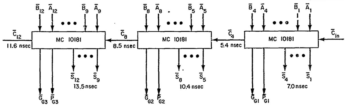
Fig. 11. 12-bit adder.
