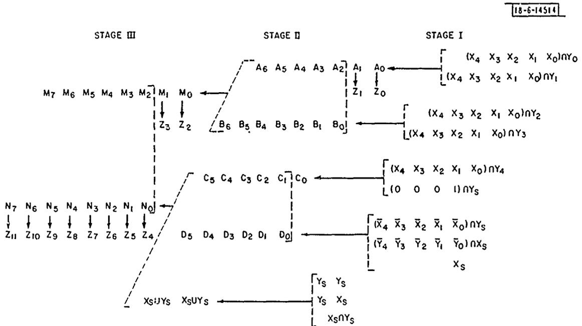
Fig. 17. Evolution of interconnections for 6 by 6 multiplier adder array.
