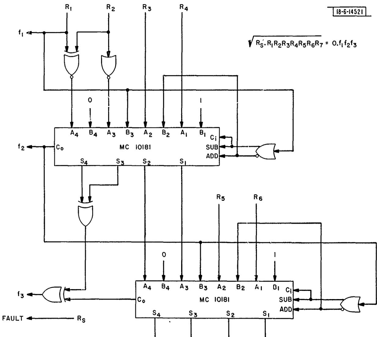
Fig. 24. Equivalent realization of 8-bit square root.
