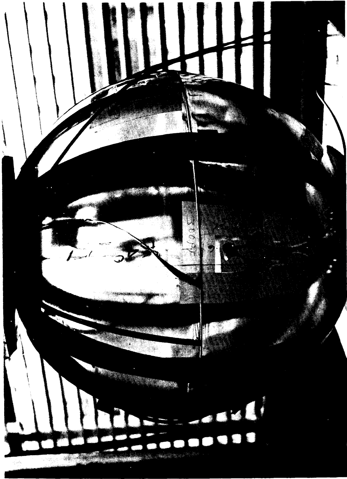
Figure 15 - Two Glass Hemispheres Subjected to Compressive Loadings
