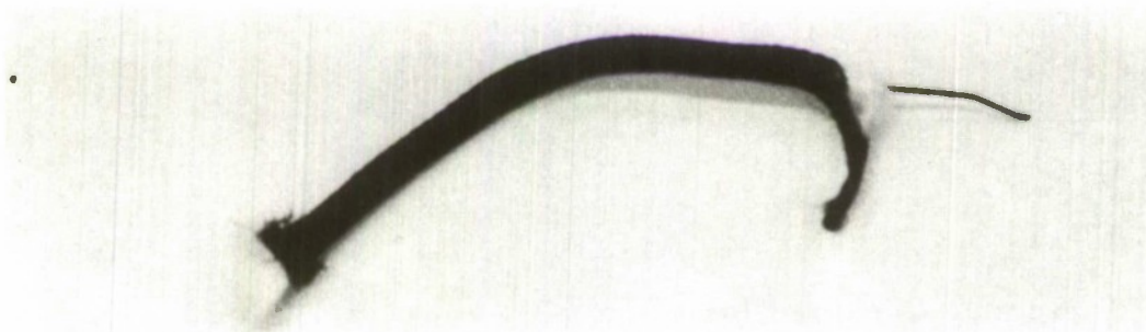
HIGH TEMPERATURE CABLE AFTER 1 HOUR AT 2000 °F—STILL FLEXIBLE
