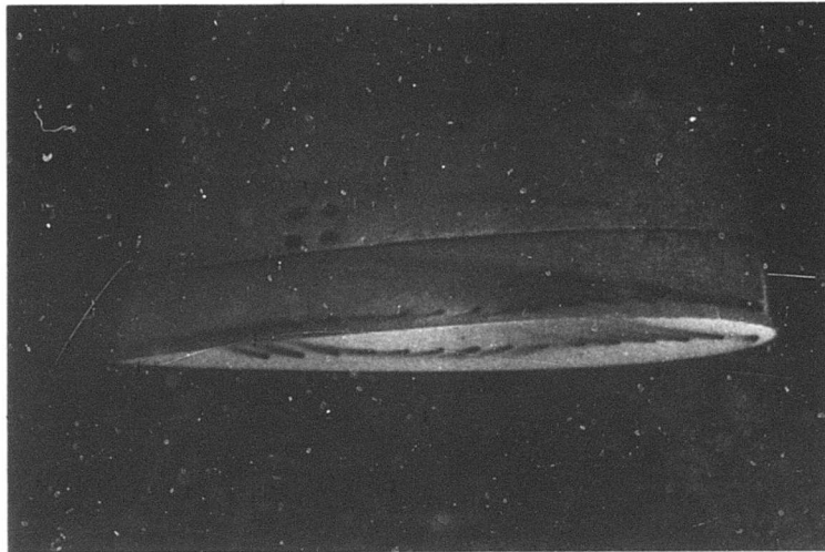
Figure 86k. Top View of Square Tip at 400 rpm and 10^\circ Pitch Angle.
