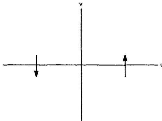
Figure 4. Ground plane replaced by dipole image.
