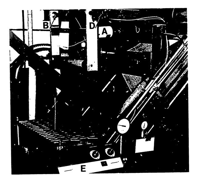
Figure 1.--Tension control device: <u>A</u>, air-cylinder spring; <u>B</u>, pivoted shaft; <u>C</u>, dancer roll; <u>D</u>, position-sensing transducer; and <u>E</u>, control box.
