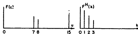
Fig. 4 a - A M-NON ZERO WALSH SPECTRUM b - ITS HADAM/ RD MBL SPECTRUM
