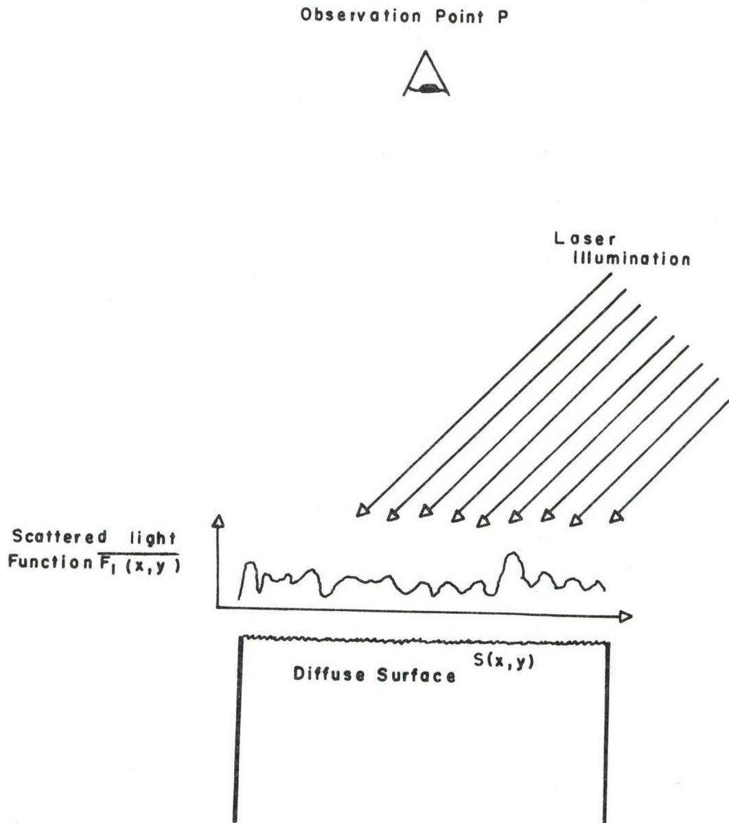
Figure 4. Configuration for Observing Speckle Pattern
