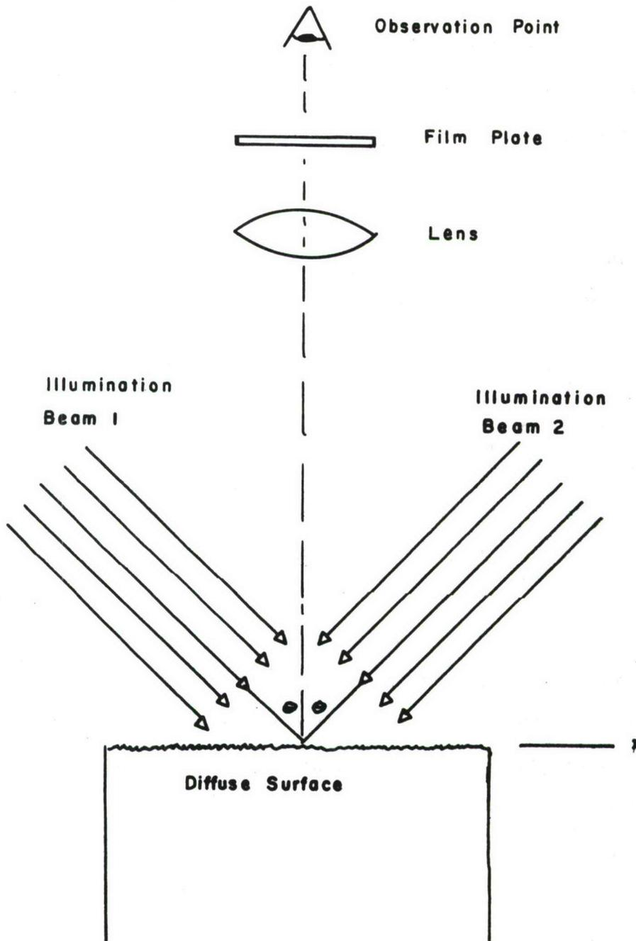
Figure 5. Experimental Configuration for Observing Speckle Correlator Fringes
