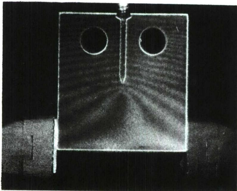
Figure 3. Speckle Correlation Fringes on Compact Tension Specimen
