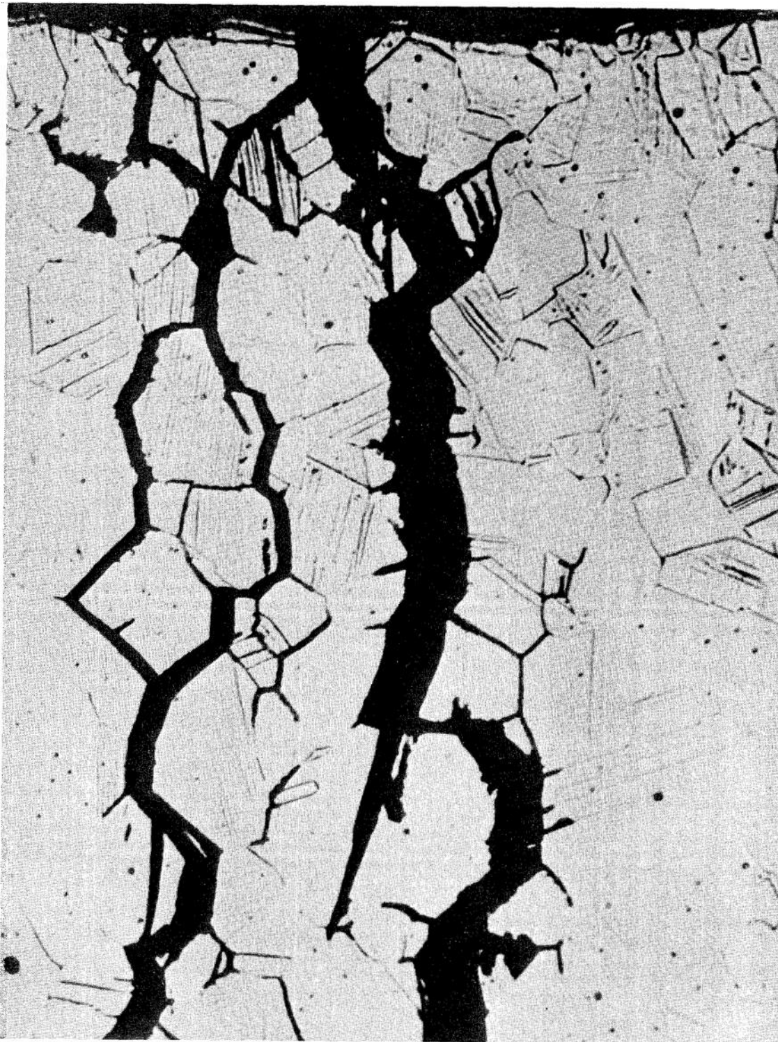
FIGURE 2: An example of complete intergranular failure in 304 stainless steel fuel element cladding. This failure occurred during irradiation in water by a mechanism akin to stress corrosion. Electrolytic oxalic acid etch.
