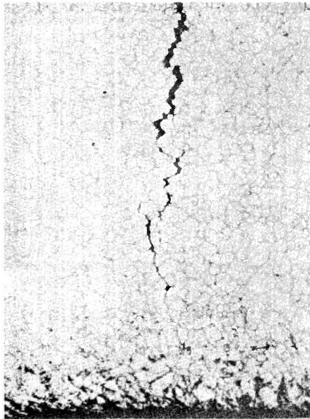
a) Intergranular Cracking of Sensitized 304 SS
