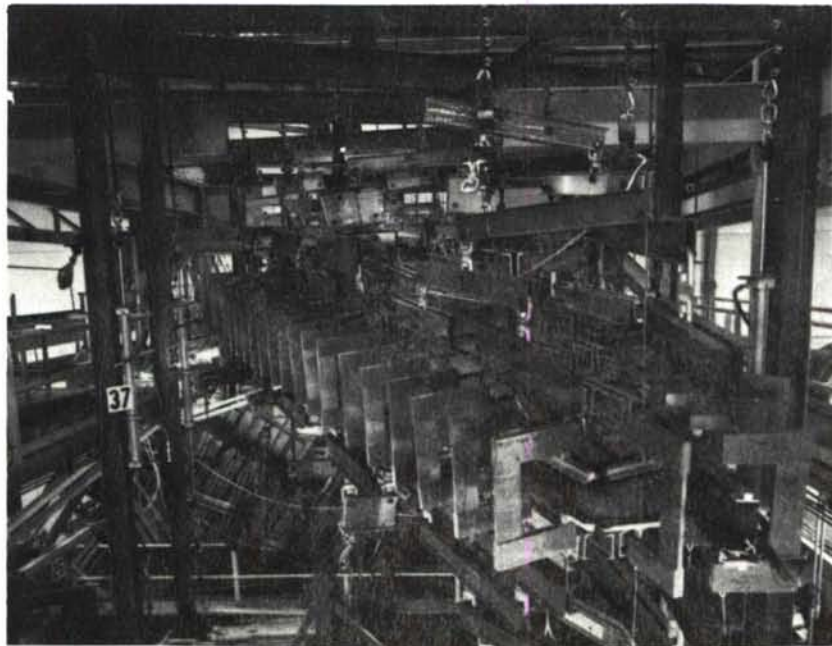
FIGURE 16. LEFT HAND HORIZONTAL STABILIZER AND SURROUNDING TEST FIXTURES. ALL SENSORS INSTALLED ON INTERNAL SURFACES
