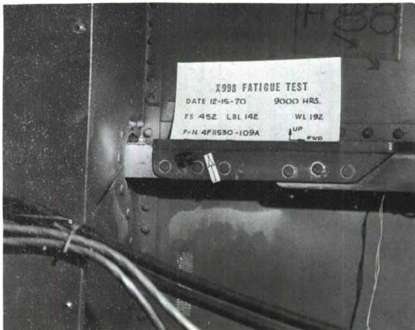
FIGURE 123. FATIGUE DAMAGE AT FUSELAGE STATION 452
