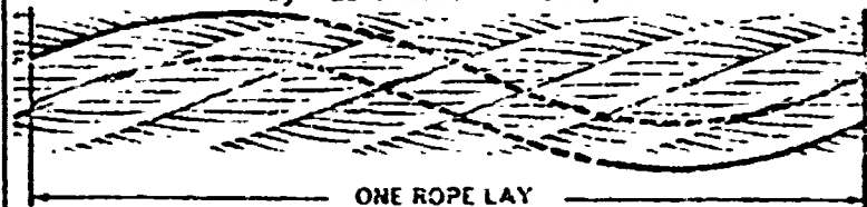
Showing how "one rope lay" is the lengthwise distance in which a strand makes one complete turn around the rope.
