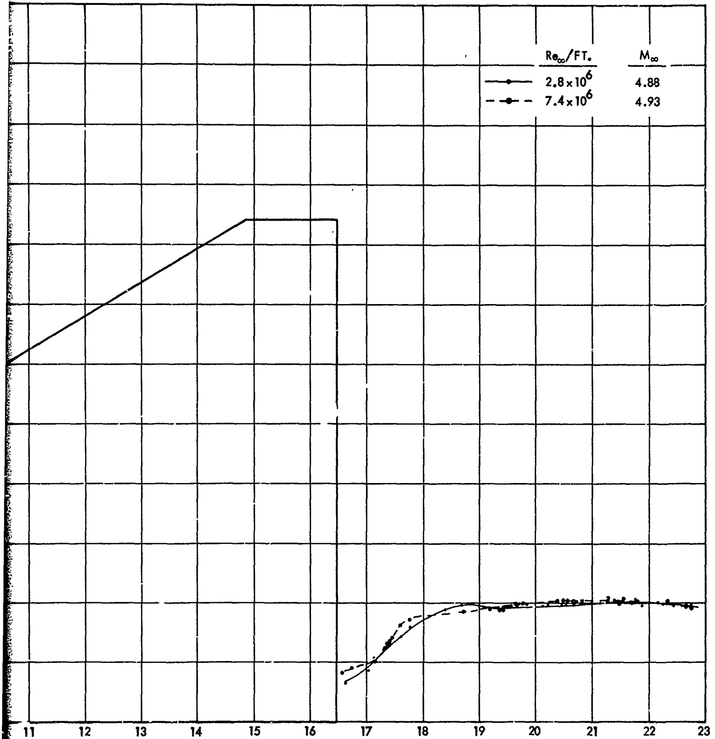
FIG. 16A FLAT PLATE PRESSURE DISTRIBUTION PRODUCED BY A 60° SWEEP FIN
