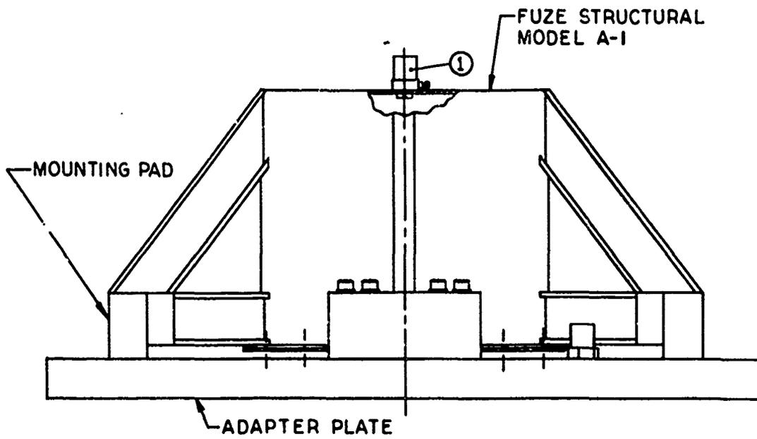
Figure 12. Fuze structural mockup A-1 on shaker adapter plate.
