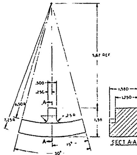
Figure 5. Aft-mounted pad.
