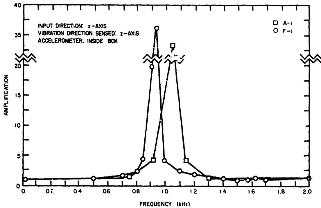
Figure 18. Response of models A-1 and F-1 to 2-g sinusoidal input.
