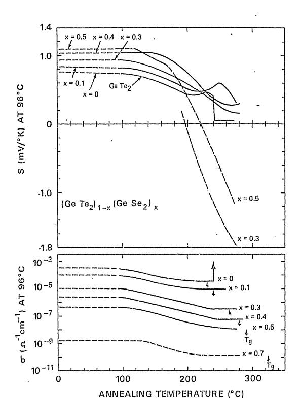
Figure 2.14 Electrical conductivity and Scebeck coefficient activation energies at  $96^{\circ}$ C versus annealing temperature for sputtered (GeTe<sub>2</sub>)  $_{1-x}$  (GeSe<sub>2</sub>)<sub>x</sub> alloys.
