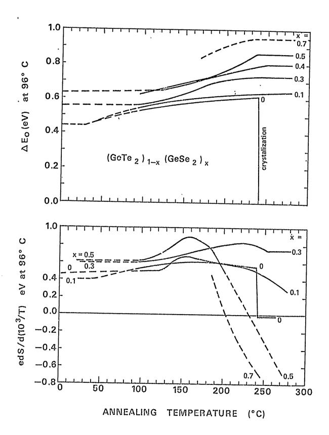
prevail in the supercooled metastable liquid state at  $\mathbf{T}_g$ . However this ordering tendency appears to be an inadequate explanation for the annealing effects which occur for both S and  $\sigma$  well below  $\mathbf{T}_g$ , due to the very low predicted atomic mobilities at these temperatures.
