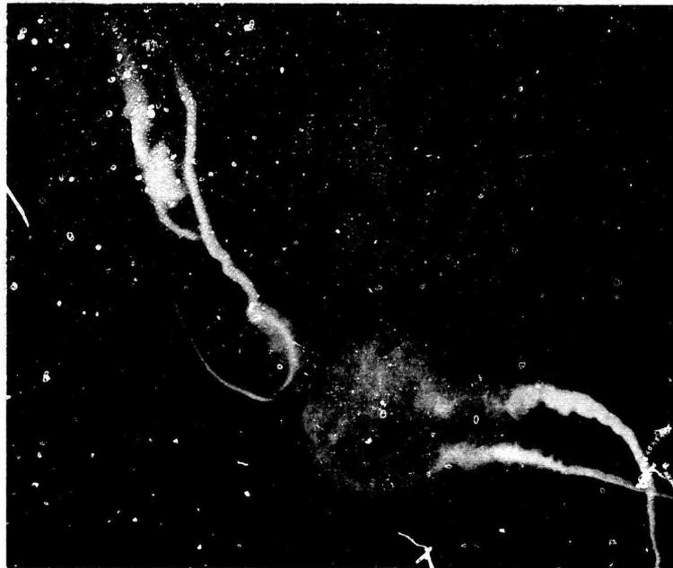
**Fig. 20. SIMULTANEOUS OCCURRENCE OF VARIOUS FORMS OF INSTABILITY. This photograph was taken from below and slightly to the side of the wake (11-4, Pass 6)**
