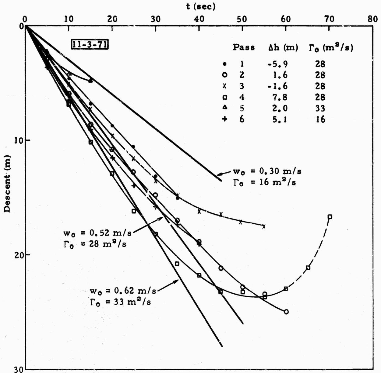
Fig. 27. TRAJECTORIES OF WAKE DESCENT IN AN ISOTHERMAL, STABLY STRATIFIED ( $\gamma \sim 0^\circ\text{C}/100$  m) ATMOSPHERE WITH NEGLIGIBLE TURBULENCE ( $\epsilon^{1/3} \sim 0.35$  cm<sup>2/3</sup>s<sup>-1</sup> FOR PASSES 1-2, 4-5) OR LIGHT TURBULENCE ( $\epsilon^{1/3} \sim 1.1$  cm<sup>2/3</sup>s<sup>-1</sup> FOR PASSES 3 AND 6)
