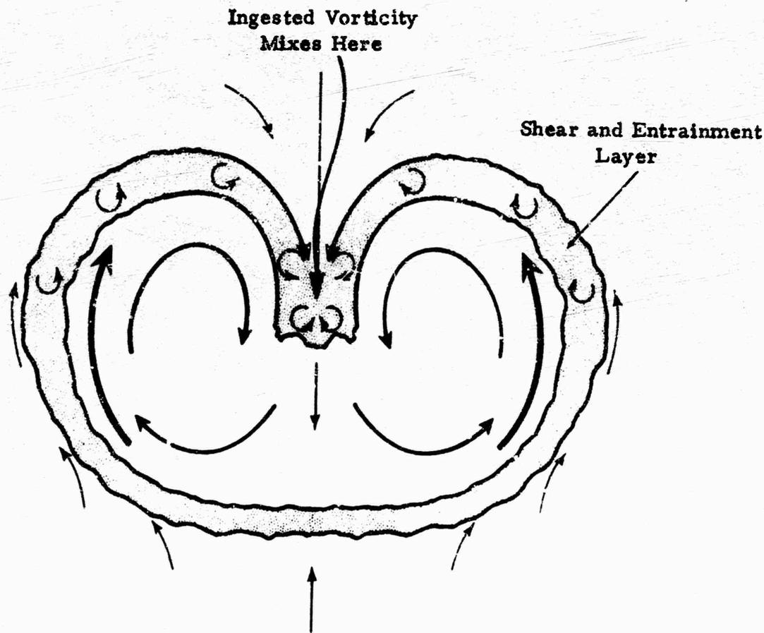
Fig. 3. MODEL OF ENTRAINING VORTEX PAIR USED BY TULIN AND SHWARTZ
