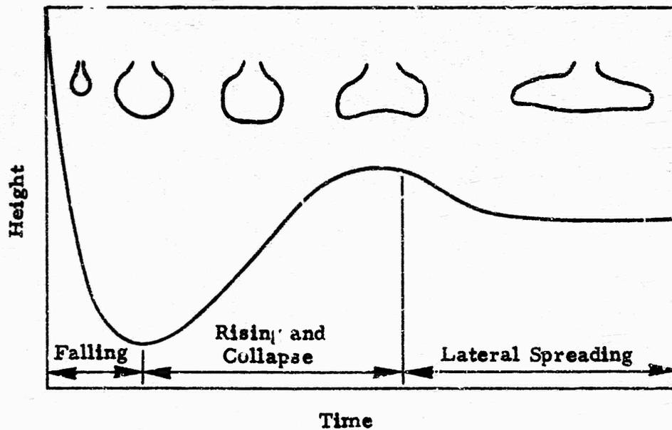
Fig. 4. TRAJECTORY OF A VORTEX PAIR IN A LINEARLY DENSITY STRATIFIED MEDIUM (from Tulin and Shwartz, 1971)
