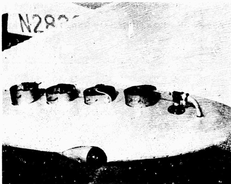
Fig. 6. MODIFIED WINGTIP FOR SMOKE GRENADE INSTALLATION
