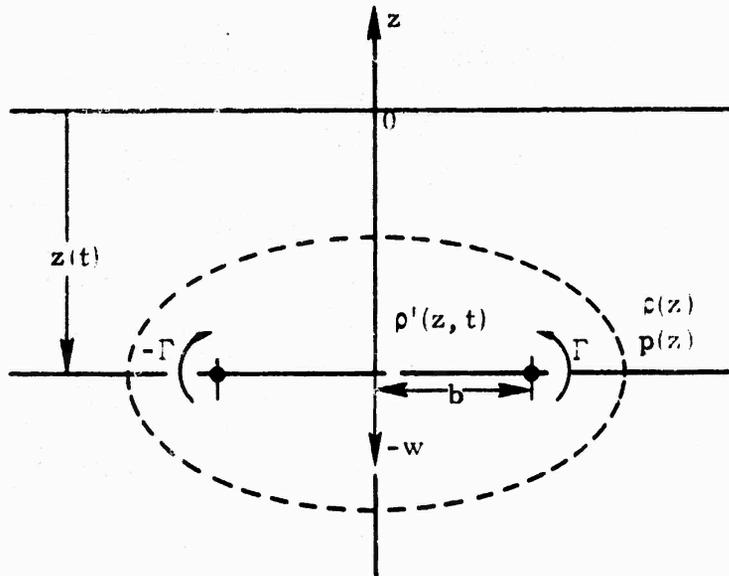
Fig. 1. Schematic cross section of vortex wake
