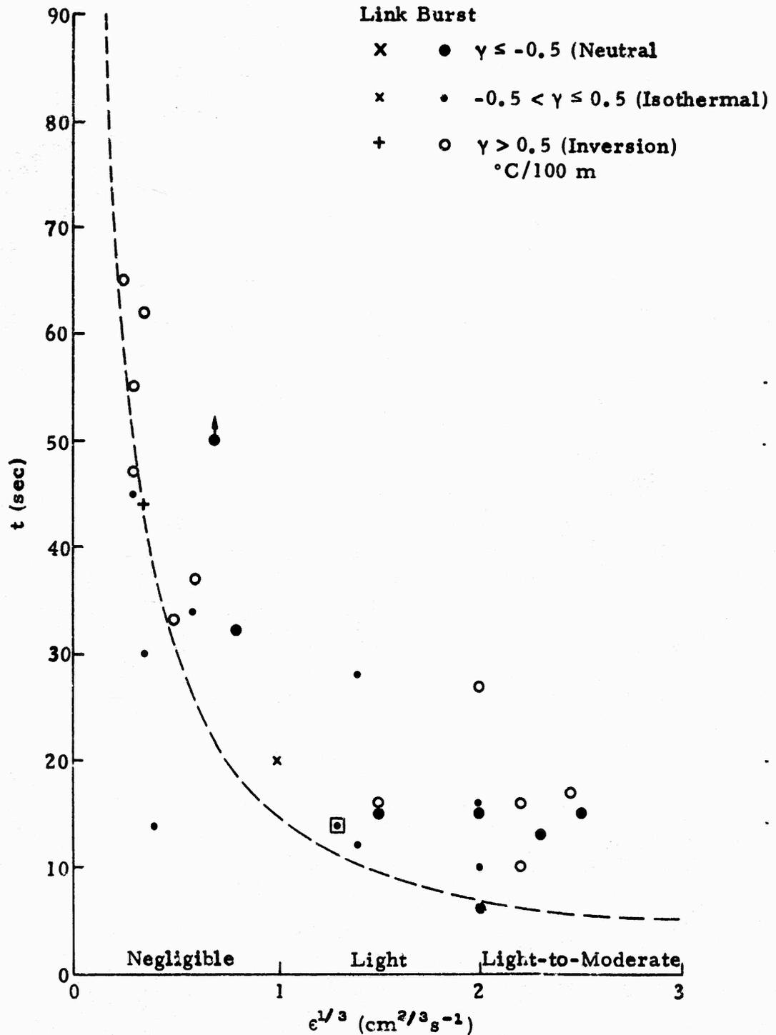
Fig. 22. PLOT OF TIME OF FIRST OBSERVED INSTABILITY AS A FUNCTION OF THE TURBULENCE LEVEL  $\epsilon^{1/3}$ . All points had  $\Gamma \sim 30 \text{ m}^2/\text{s}$  except for the one point marked  $\square$ , where  $\Gamma = 16 \text{ m}^2/\text{s}$ . An early bound to the data is shown. The point with an arrow indicates that an instability had not appeared at the indicated time but that data for a longer time is not available.
