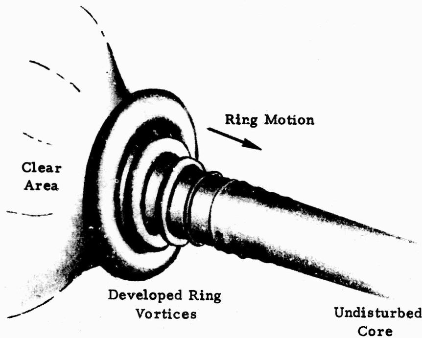
Fig. 15. SCHEMATIC REPRESENTATION OF POSSIBLE CORE BURST CONFIGURATION
