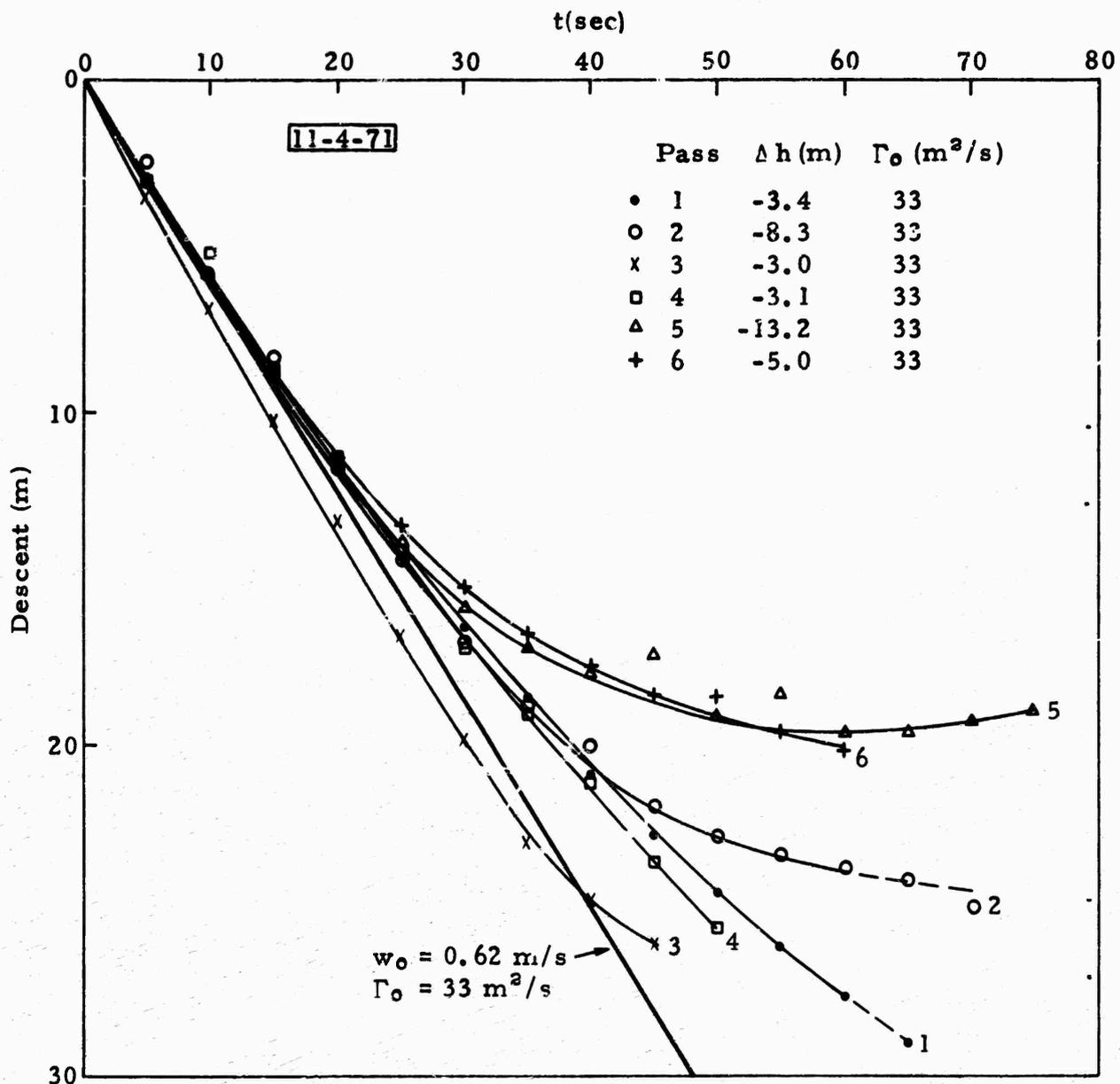
Fig. 26. TRAJECTORIES OF WAKE DESCENT IN A STABLY STRATIFIED ATMOSPHERE ( $\gamma \sim 1^\circ\text{C}/100 \text{ m}$ , AN INVERSION) WITH NEGLIGIBLE TURBULENCE ( $\epsilon^{1/3} \sim 0.3 \text{ cm}^{2/3}\text{s}^{-1}$ )
