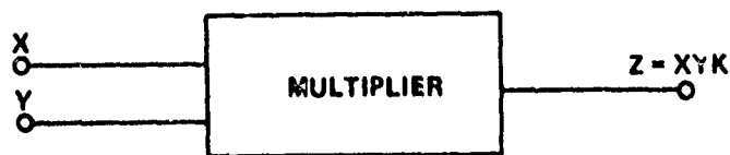
Figure 7. Functional Diagram of an Electronic Multiplier
