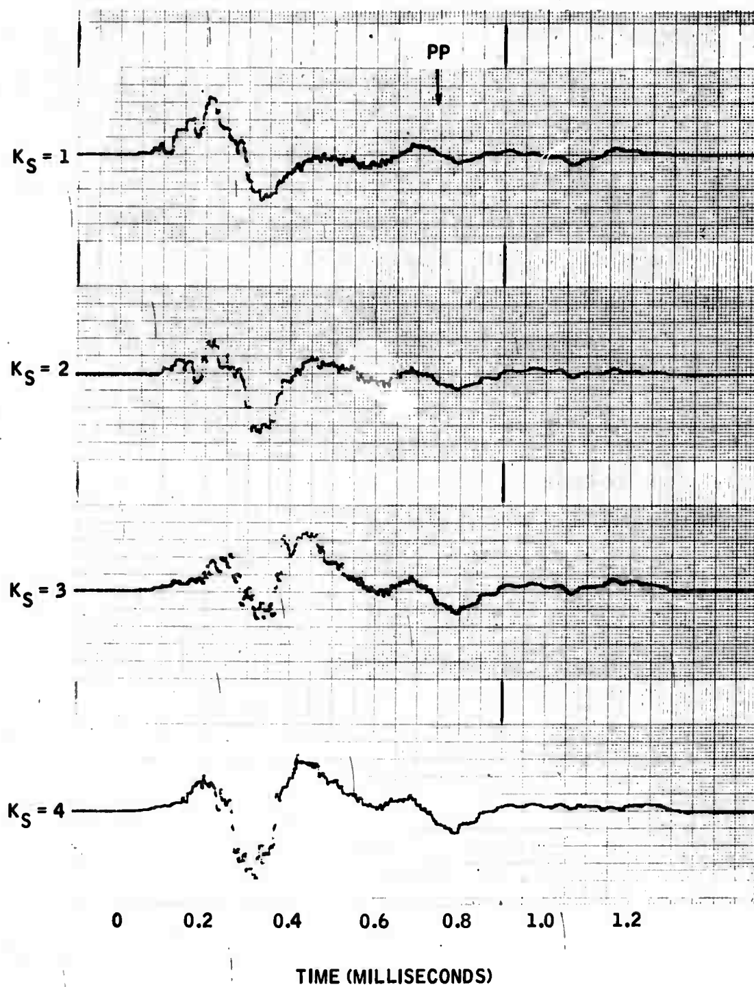
Figure 4-42. Granite Block, Cross-Correlation (SXU) of Fan Filter Ten-Element Beams
