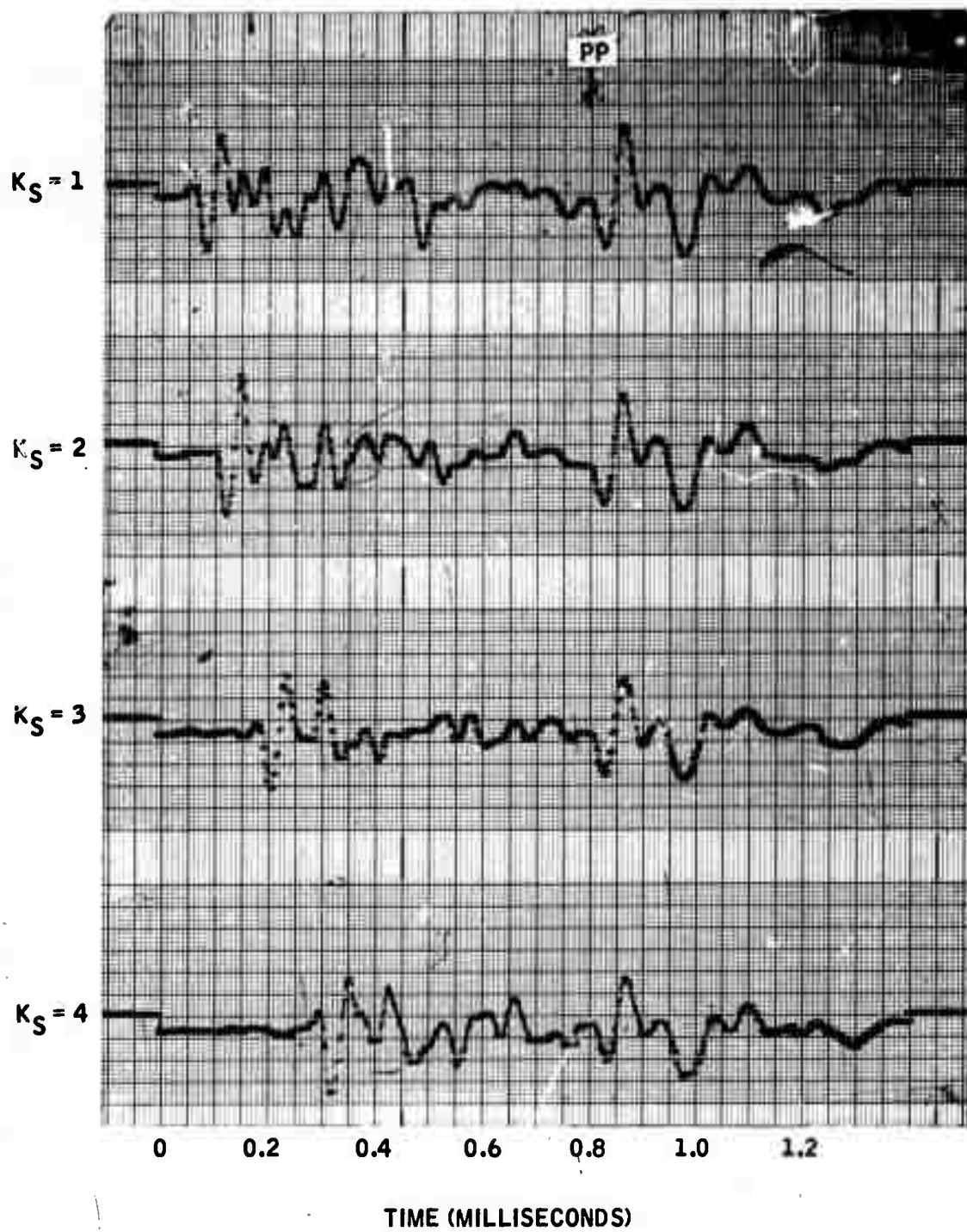
Figure 4-17. Seismic Model, Ten-Element Delay-and-Sum Beamformer
