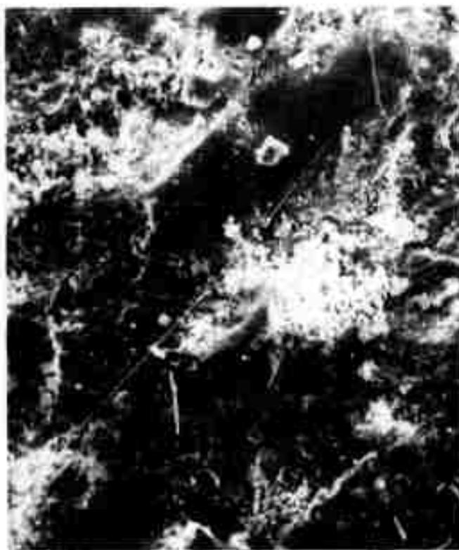
Fig. 5. Scanning electron micrograph of surface after completion of sliding. Note debris. Test 100C,  $\sigma_n = 20 \text{ kg/cm}^2$ , 300X.
