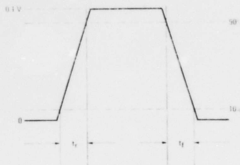
FIGURE 3 — PULSE RESPONSE TEST WAVEFORM
