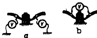
Figure 3. Testing the connecting resistance at a terminal by comparing two readings on a voltmeter (a), and by direct measurement (b)
