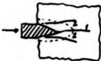
Fig. 1. Nature of Ice's Breakdown by Bridge Pier with Sloped Edge: 1-leading cracks; and 2-ice projections.
