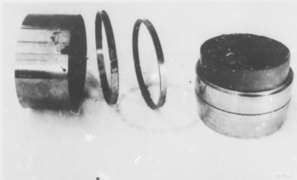
Figure A.16 3.6-inch-diameter ring sampler after removal of driving sleeve, small support sleeve, and upper collar.
