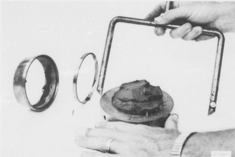
Figure A.19 3.6-inch-diameter specimen being trimmed flush with container ring and test device adapter after removal of cutting shoe, large support sleeve, and lower collar.
