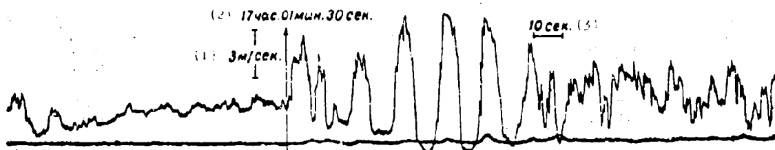
Fig. 6.8. Segment of recording of an airborne hot-wire anemometer showing wave perturbations (per N. K. Vinnichenko).
