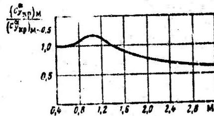
Figure 9.9. Mach-number plot of the ratio  $(c_{y_{wg}}^\alpha)_M / (c_{y_{wg}}^\alpha)_{M \leq 0.5}$ .
