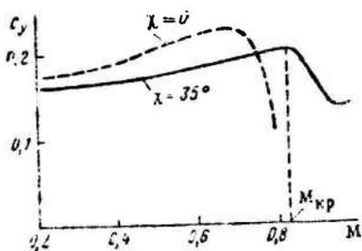
Figure 8.13. Coefficient  $c_y$  as a function of  $M$  (at  $\alpha = 2^\circ$ ) for swept and unswept wings built up from identical profiles.
