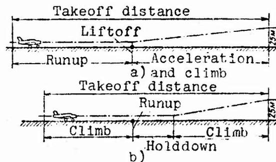
Figure 7.1. Diagrams of takeoff: a) turbojet airplane; b) propeller-driven airplane (with low power/weight ratio).
