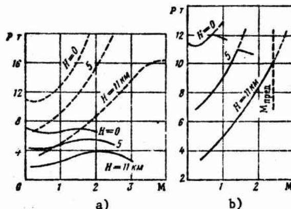
Figure 4.14. a) Thrust of TJE as function of  $M$  and altitude. Solid line: engine thrust without augmentation; dashed line: with augmentation; b) thrust of TJE with augmentation as a function of  $M$  and altitude. Solid line: strength limitations; dashed line: thrust without these limitations.
