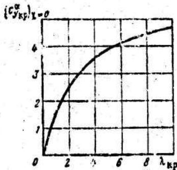
Figure 9.8. The derivative  $(c_{y_{wg}}^\alpha)_{\chi=0}$  for straight (unswept) wing as a function of aspect ratio  $\lambda_{wg}$  at  $M \leq 0.5$ .
