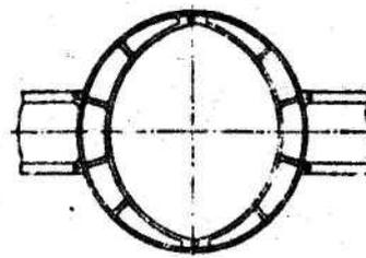
Figure 12.29. Transmission of moment across annular bulkhead.
