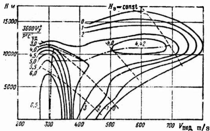
Figure 6.12. Diagram for determining rate of climb that ensures reaching energy altitude with minimum fuel consumption.
