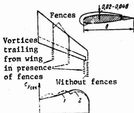
Figure 8.7. Effect of mounting stall fences\* on upper surface of swept wing on spanwise distribution of the lift coefficient  $c_{y \text{ sec}}$ :
