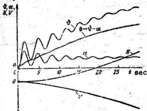
Figure 6.32. Variation of longitudinal-motion parameters of airplane after an instantaneous deflection of the stabilizer by a constant amount  $\Delta\phi_{st} = -1^\circ$ .
