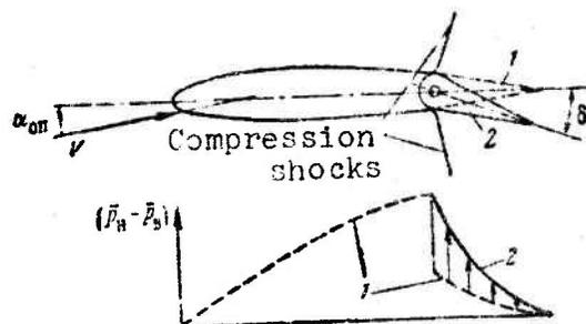
Figure 8.19. Schematic drawing of change in aerodynamic load on tail surface in transonic flow ( $M > M_{cr}$ ):
