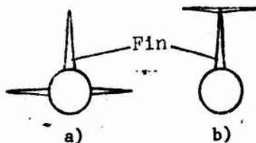
Figure 8.11. Diagrams showing two placements of horizontal tail to obtain minimum downwash in the symmetry plane of the airplane: a) horizontal tail on fuselage; b) horizontal tail on vertical fin.
