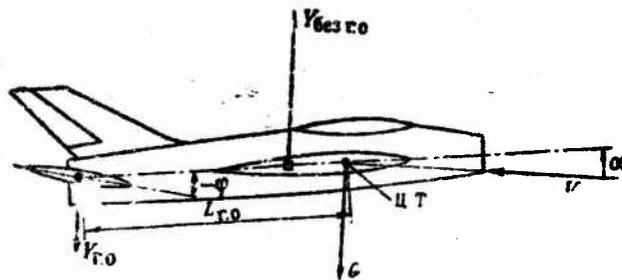
Figure 8.24. Longitudinal balance of airplane of conventional configuration.
