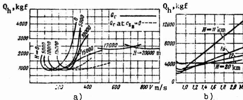
Figure 4.9. a)  $Q_h$  as a function of speed and altitude; b)  $Q_h$  as a function of  $M$  and altitude.
