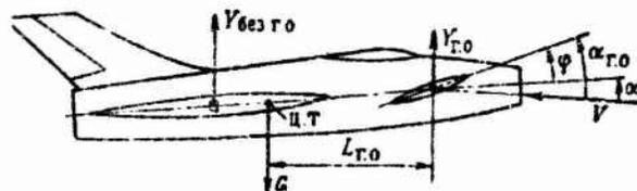
Figure 8.25. Longitudinal balance of airplane of "canard" configuration.
