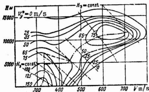
Figure 5.15. Diagram for calculation of  $V_{clb}$  as a function of altitude to ensure fastest climb to energy altitude.
