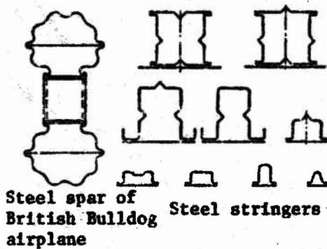
Figure 12.19. Cross sections of steel spar and stringers.
