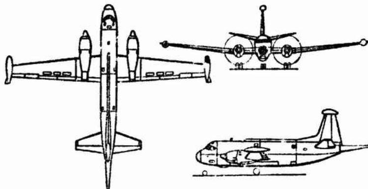
Figure 14.9. Breguet Atlantique antisubmarine airplane.  $G = 43,500$  kg,  $S = 120$  m<sup>2</sup>,  $H_{olg} = 9,100$  m. Maximum endurance 18 h.
