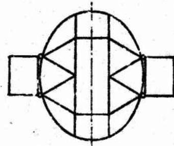
Figure 13.2. Tail bulkhead with aisle and pylons.
