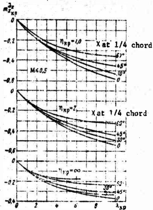
Figure 9.22. Derivatives  $m_{\dot{\omega}_x}^{xWG}$  of isolated wings as functions of their aspect ratio  $\lambda_{WG}$  at  $M \leq 0.5$ .
