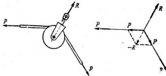
Figure 12.5. Control pulley.
