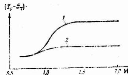
Figure 8.28. Mach-number curves of normal-acceleration stability of aircraft with fixed (1) and in-flight-variable (2) tailplanes.
