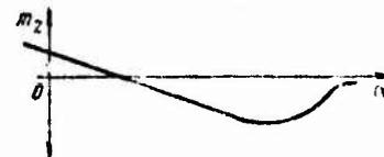
Figure 8.4. Pitching-moment-coefficient variation of a swept-wing airplane as a function of angle of attack.
