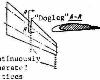
Figure 8.10. Diagram of "dogleg" on leading edge of swept wing.
