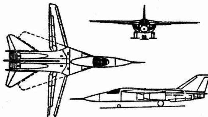
Figure 14.2. Dynamics Grumman F-111A multi-purpose fighter-bomber.  $G = 32,000$  kg,  $S = 57-64$  m<sup>2</sup>,  $P_{11} \approx 24,400$  kgf,  $M_{lim} = 2.5$ ,  $H_{clg} = 18,000-19,000$  m.
