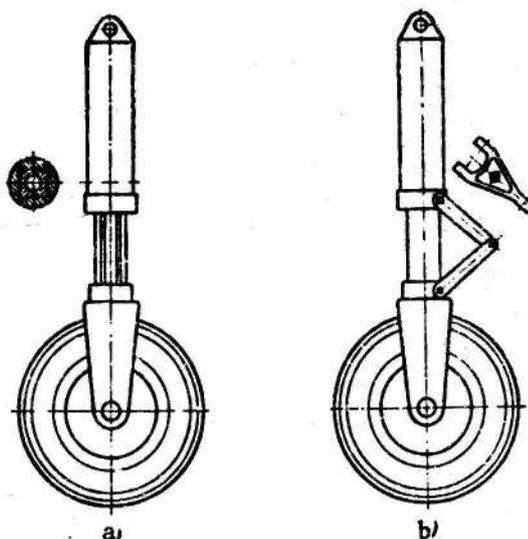
Figure 1.2. Landing-gear strut. 1) with spline; b) with torque arms.
