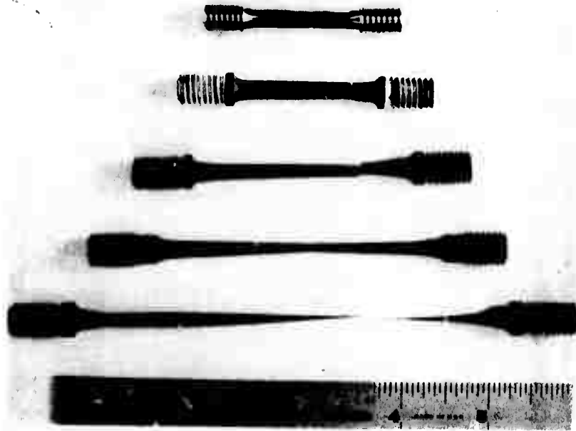
Figure 11 - As-extruded tensile bars superplastically deformed at 1900°F at indicated strain rates.
