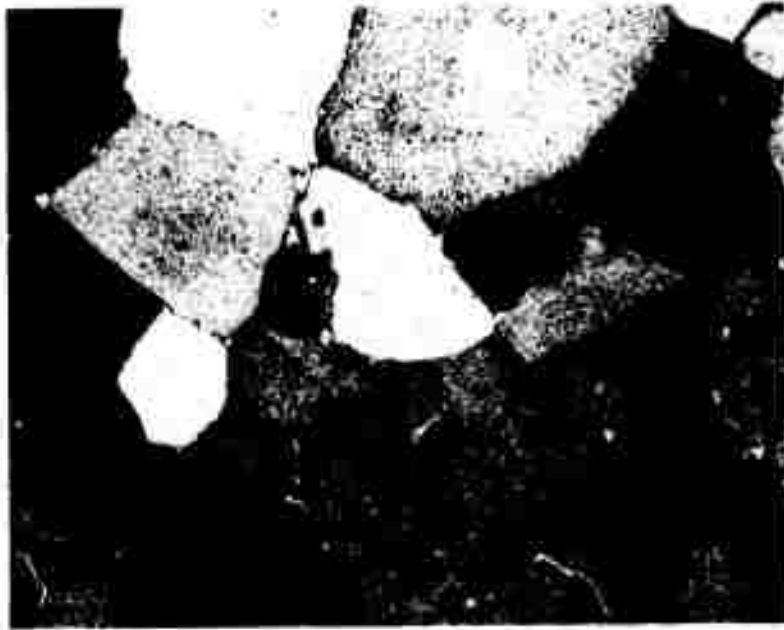
Figure 7. IN-100, low carbon, R.E.P. powder, -35 mesh. HIP @ 2300° F, 27,700 psi, 1 hr. As pressed. Etched. 100X.
