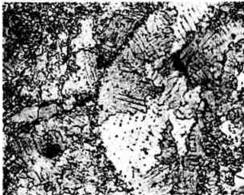
Figure 6. IN-100, low carbon, R.E.P. powder, -35 mesh. HIP @ 1825°F, 27,700 psi, 1 hr. As pressed. Etched. 1000X.
