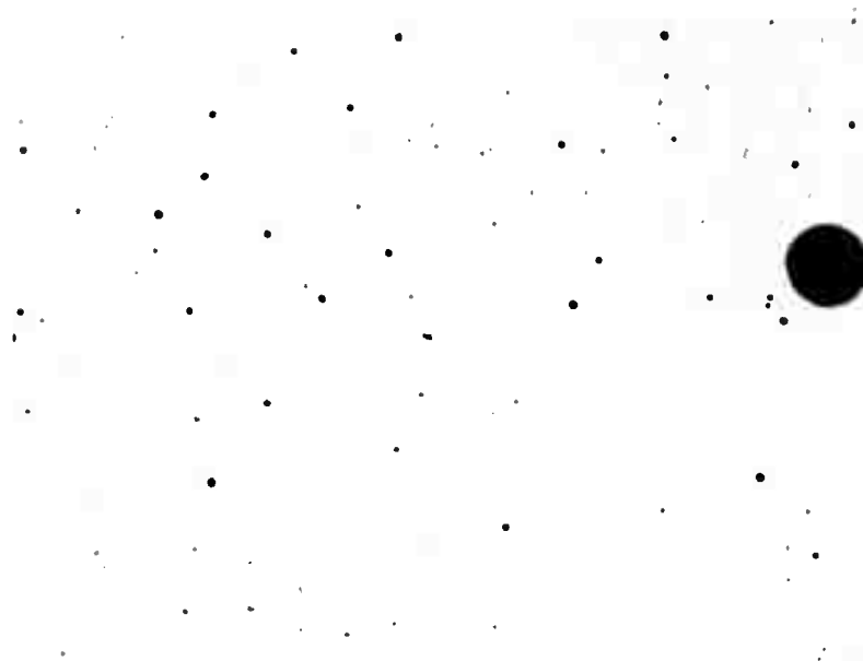
Figure 3. Ni-Co-Mo maraging steel. Heat No. 231. -8/+10 mesh. Oxide inclusions. Unetched. 500X.
