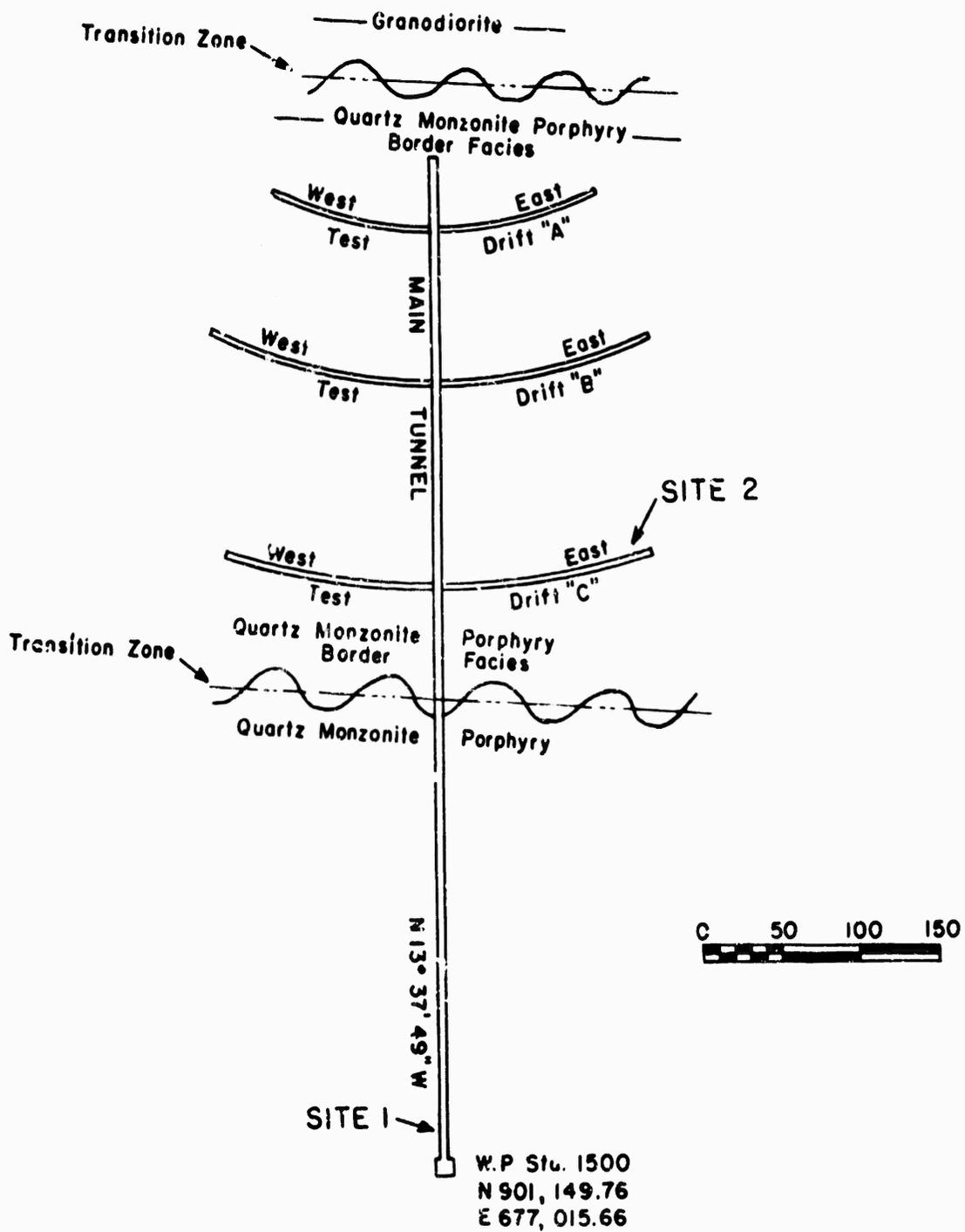
Figure 1 Plan of Hard Hat excavation.
