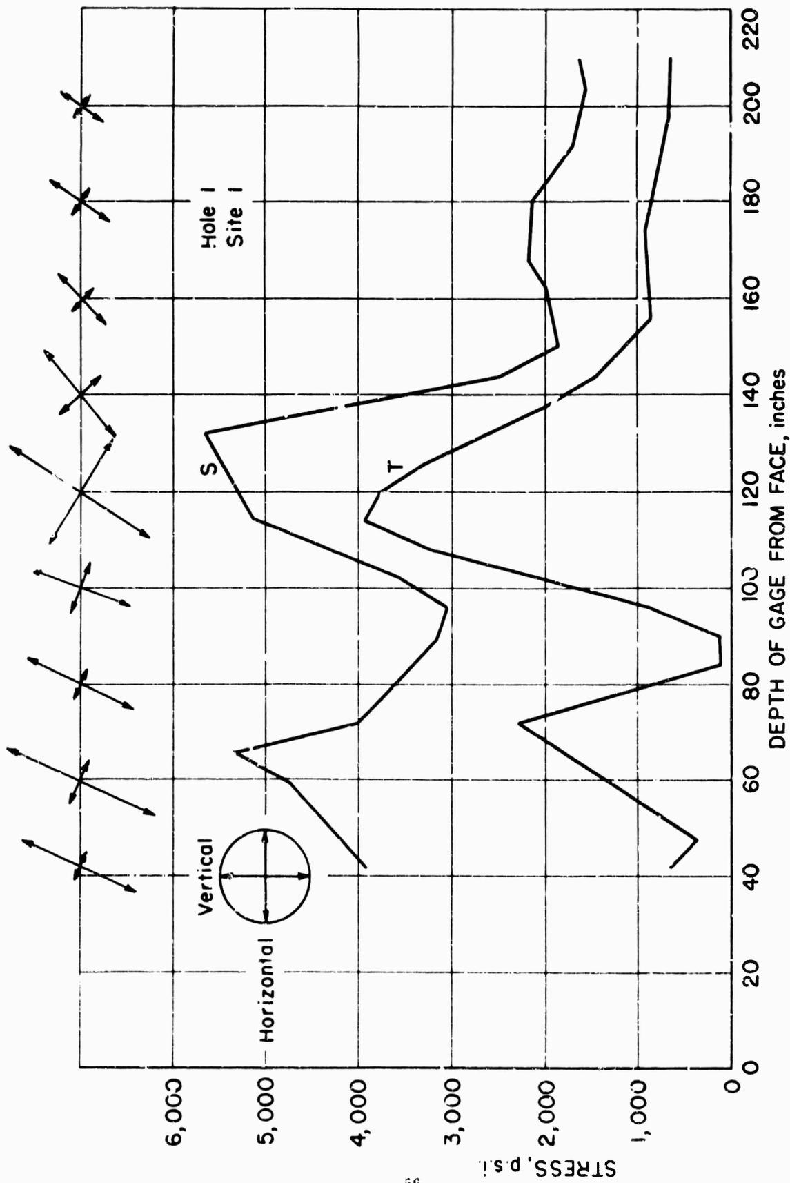
Figure 17 Stress versus depth of gage, Site 1, Hole 1.
