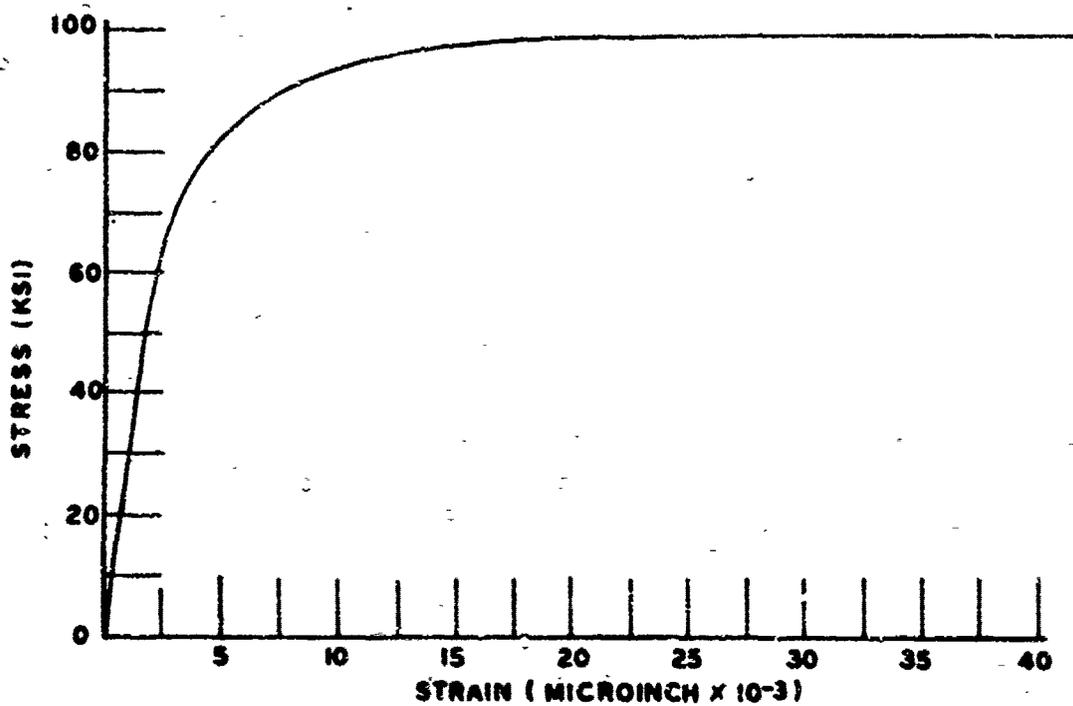
Figure 9. XY Plotter Results, Steel Tensile Specimen, S2
