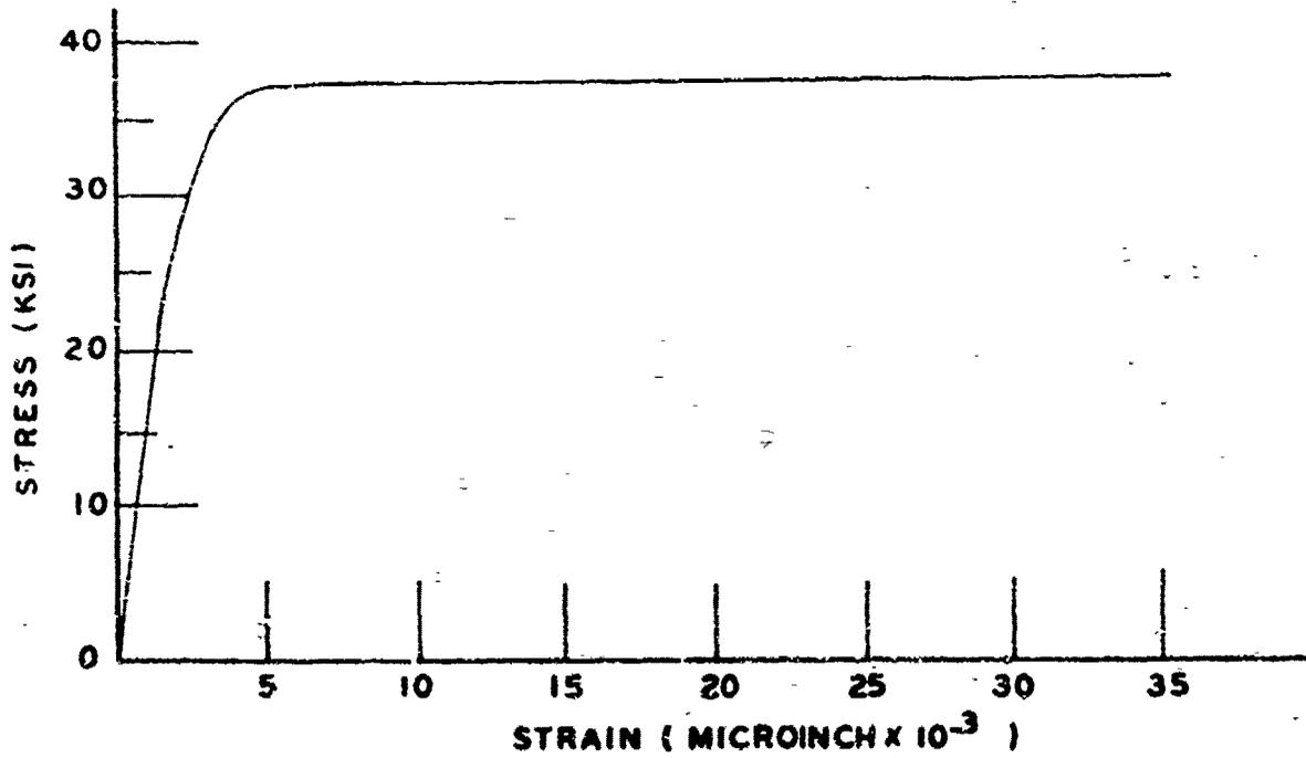
Figure 7. XY Plotter Results, Copper Tensile Specimen, C1
