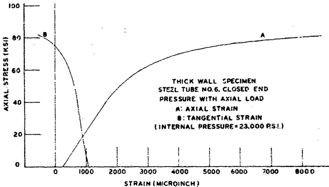
Figure 17. Steel Closed End with Axial Load
