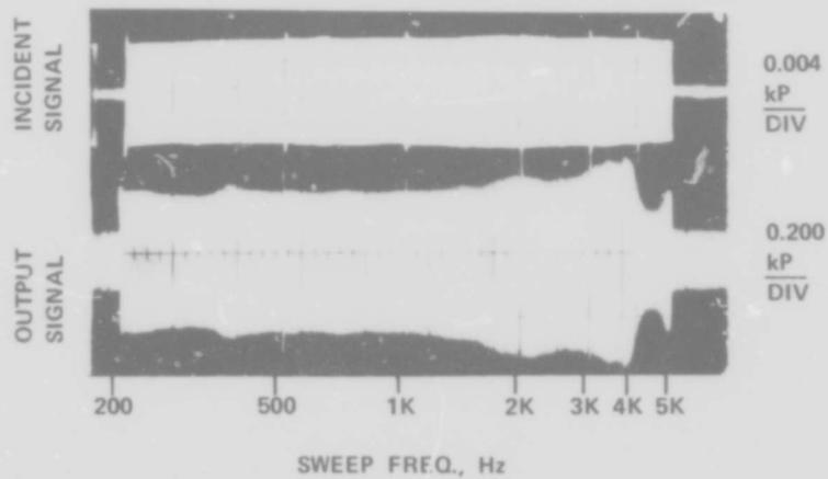
Figure 8. Frequency response of five-stage amplifier with power-jet pressure of 50 kP.
