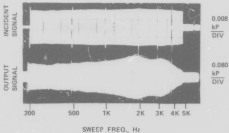
Figure 9. Frequency response of three-stage amplifier with power-jet pressure of 75 kP.
