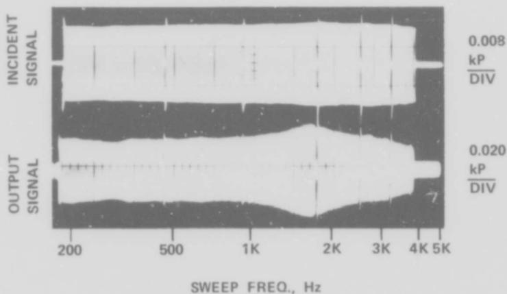
Figure 11. Frequency response of one-stage amplifier with power-jet pressure of 10 kP.
