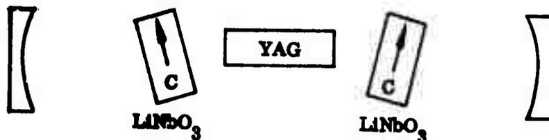
Fig. 2-15 Arrangement Used for Demonstrating Electrooptic Elimination of Spatial Hole Burning. Two lithium niobate crystals with their c-axes as shown are modulating the phase of the standing wave pattern in the rod
