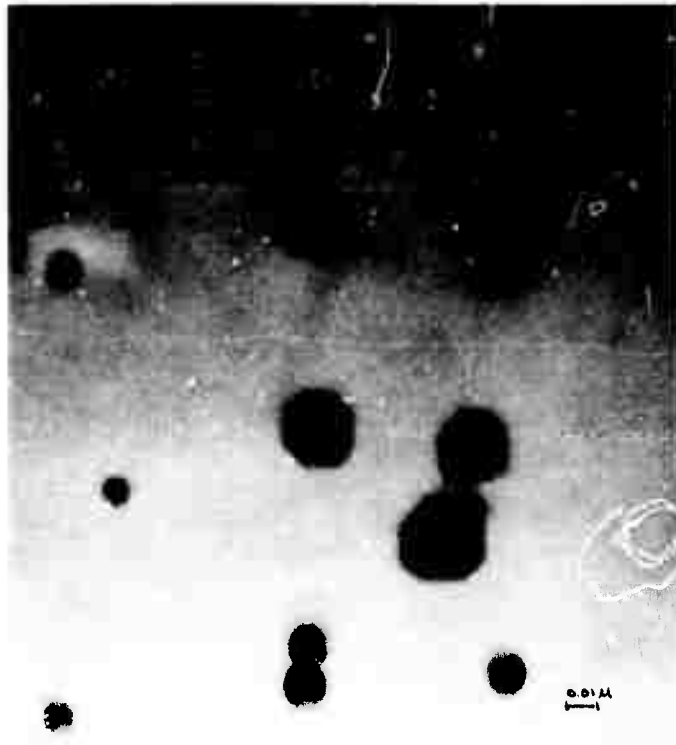
Figure IV-1. Multi-faceted polyhedra precipitates.
