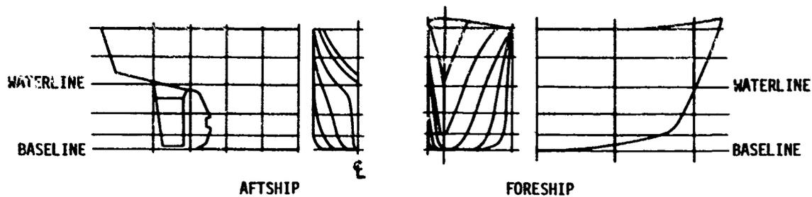
Figure 1 - Hull Lines of Catamaran Model 5061
