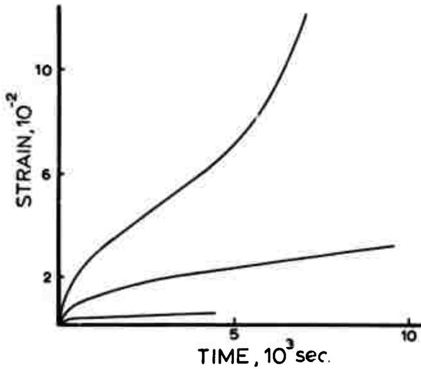
FIGURE 1. Creep curves of Solenhofen limestone subjected to different shear stresses at 150,000 psi confining pressure (after Griggs)
