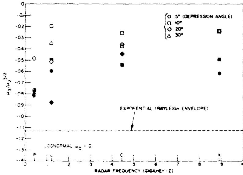
Fig. 16—Third central moment of sea clutter taken with the 4FR system for rough seas. The wind speed was 15 to 20 meters/second. The solid points represent vertical polarization and the open points, horizontal polarization.
