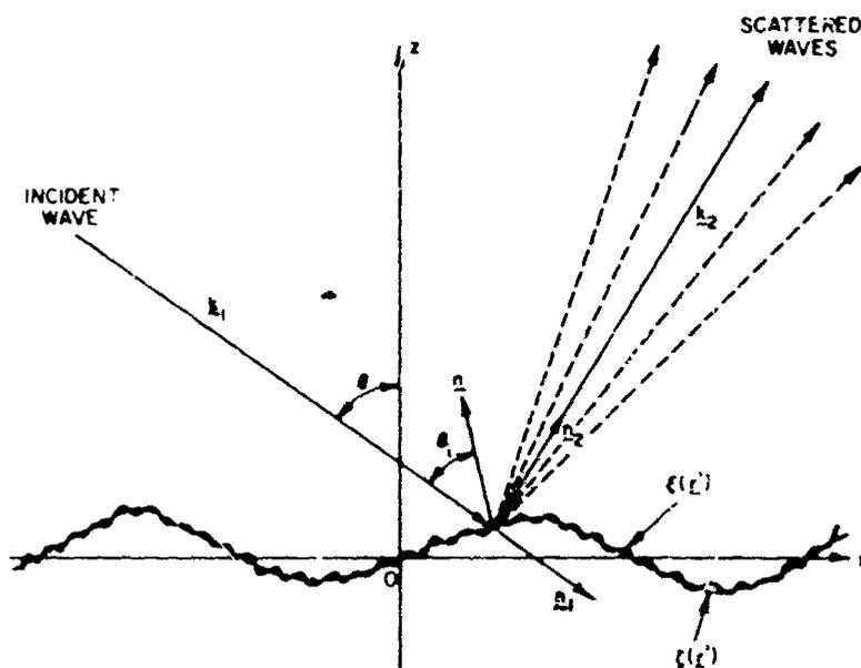
Fig. 1—Scattering geometry
