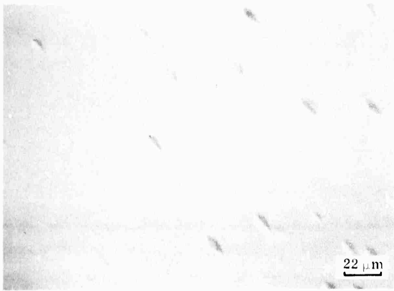
Figure 4. Surface Structure of (10\bar{1}4) Al_2O_3 after Removal \sim 7 \mu m of Al_2O_3 by Freon Etch at 1550 C (Etch Rate \sim 0.1 \mu m/min )
