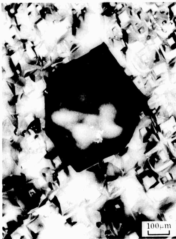
Figure 5. The Surface of Verneuil-Grown (10\bar{1}4) Al_2O_3 after Etching with Freon at 1500 C for \sim 3 Hr at Nominal Rate of 0.6 \mu\text{m}/\text{min} . Several Deep Large Etch Pits (as in Center) were Randomly Distributed on Surface.
