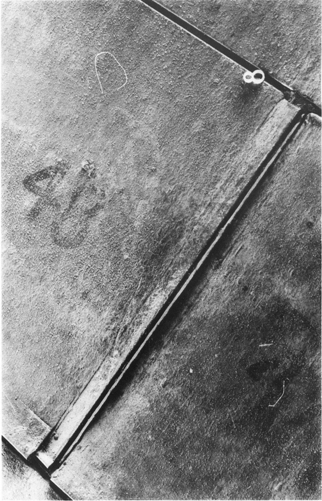
Photograph 8. Sheared end joint in item 2 after 150 coverages of 27,000-lb single-wheel load
