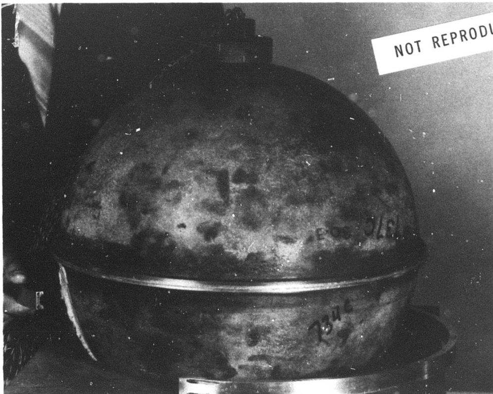
Figure 3. Assembly of sphere F with an aluminum joint.
