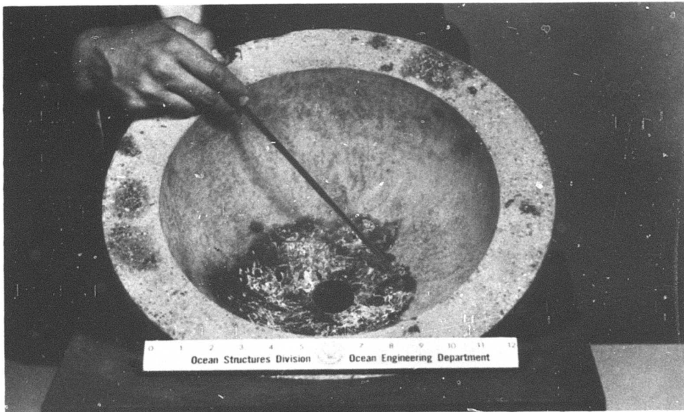
Figure 2. Appearance of concrete hemisphere after impregnation with DAP monomer.
