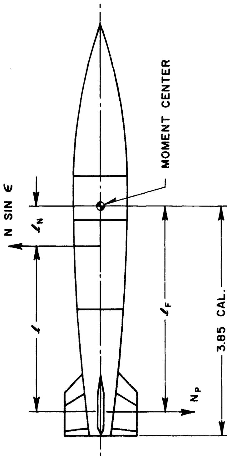
Figure 3. The Couple Created by Normal Force Interaction
