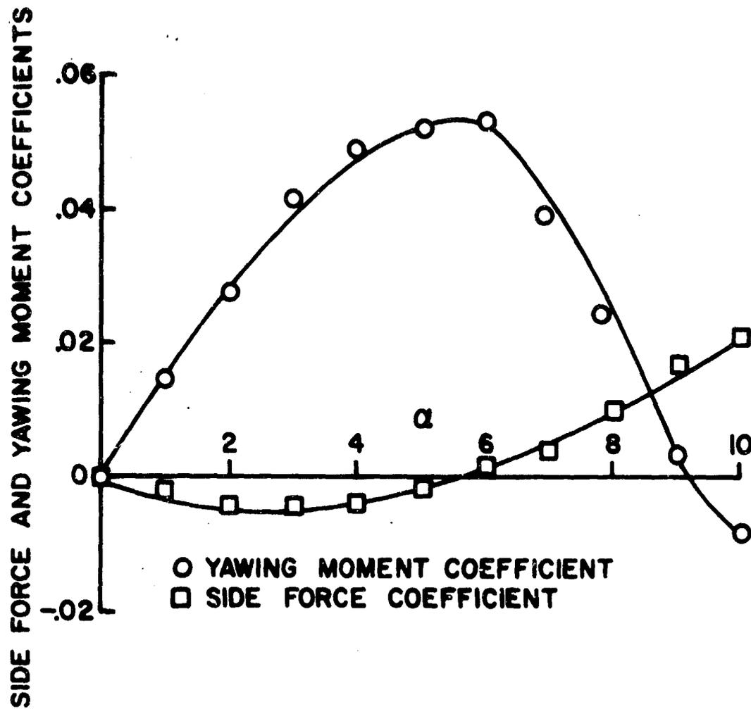
Figure 2. Side Force and Yawing Moment Coefficients Versus Angle of Attack for a 4° Fin Cant at Mach Number 0.90,  $Re = 1.5 \times 10^6$
