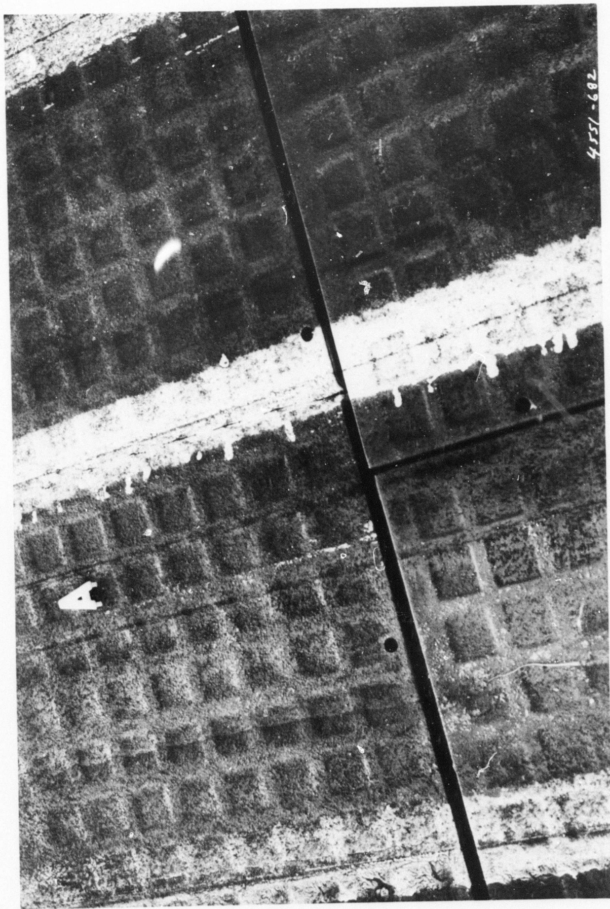
Photograph 9. Close-up of panel 17 in item 1 showing shear in facing at 200 coverages
