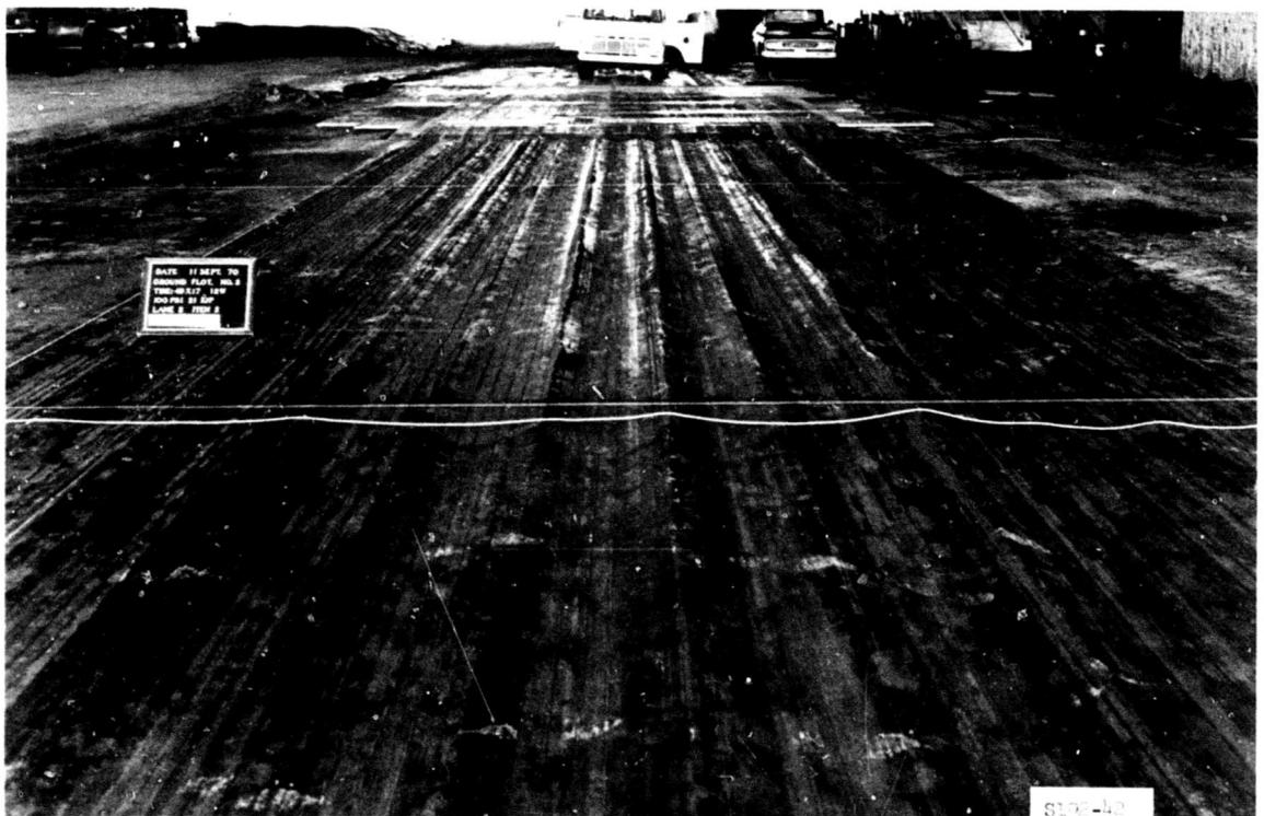
Photo 16. Test section 2, lane 2, item 2, at failure after 76 coverages
