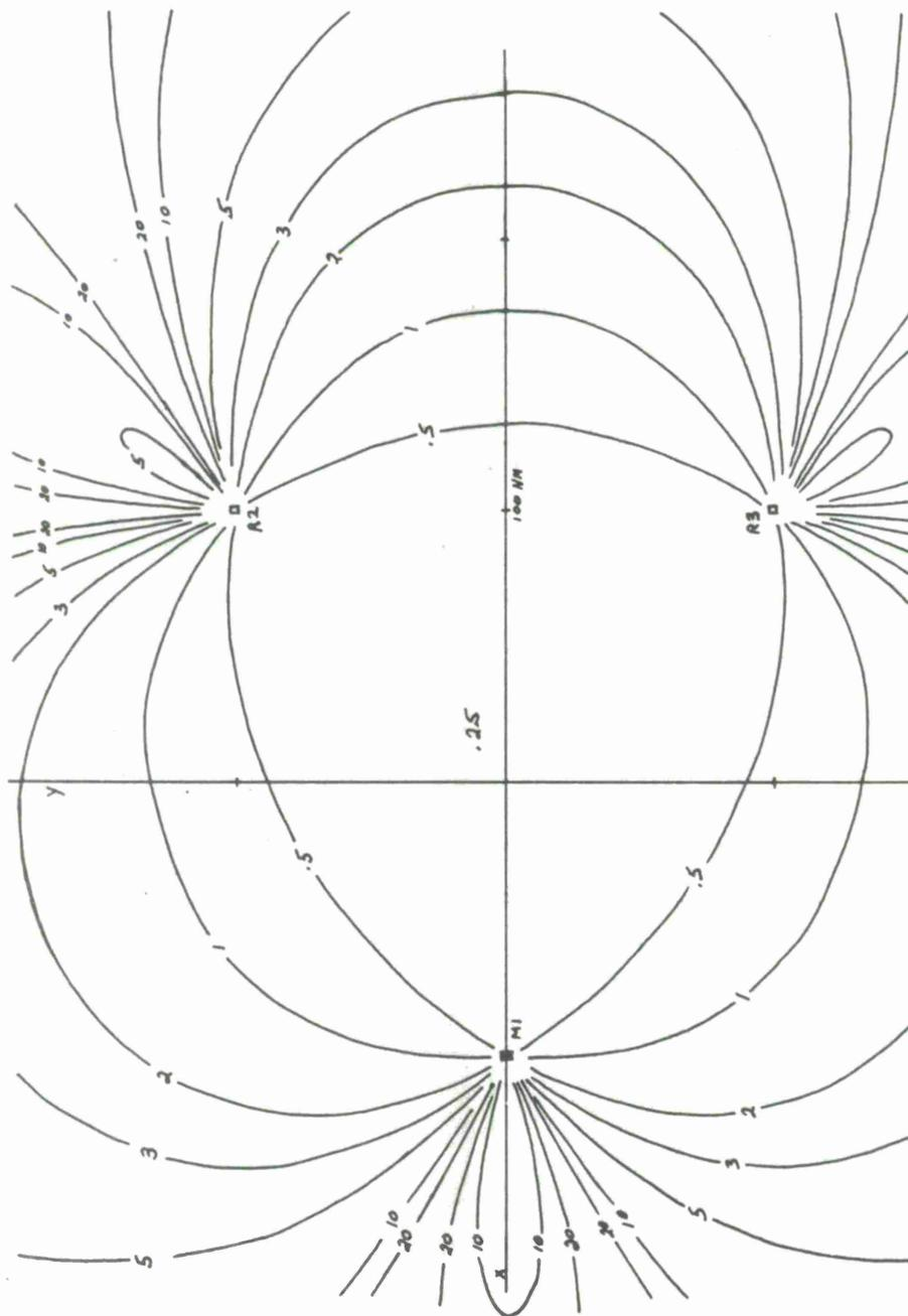
Figure 40. Geometric Dilution of Precision--Single Fix, Time. Five Reports per Frame from Each of Three Perfect References. Showing  $\sigma/\omega$  versus  $x, y$ .
