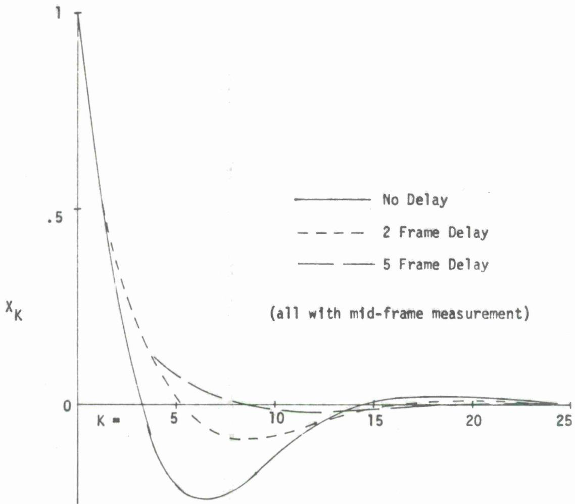
Figure 9. Effect of Delay in Rate Adjustment on Unit Position Step Response
