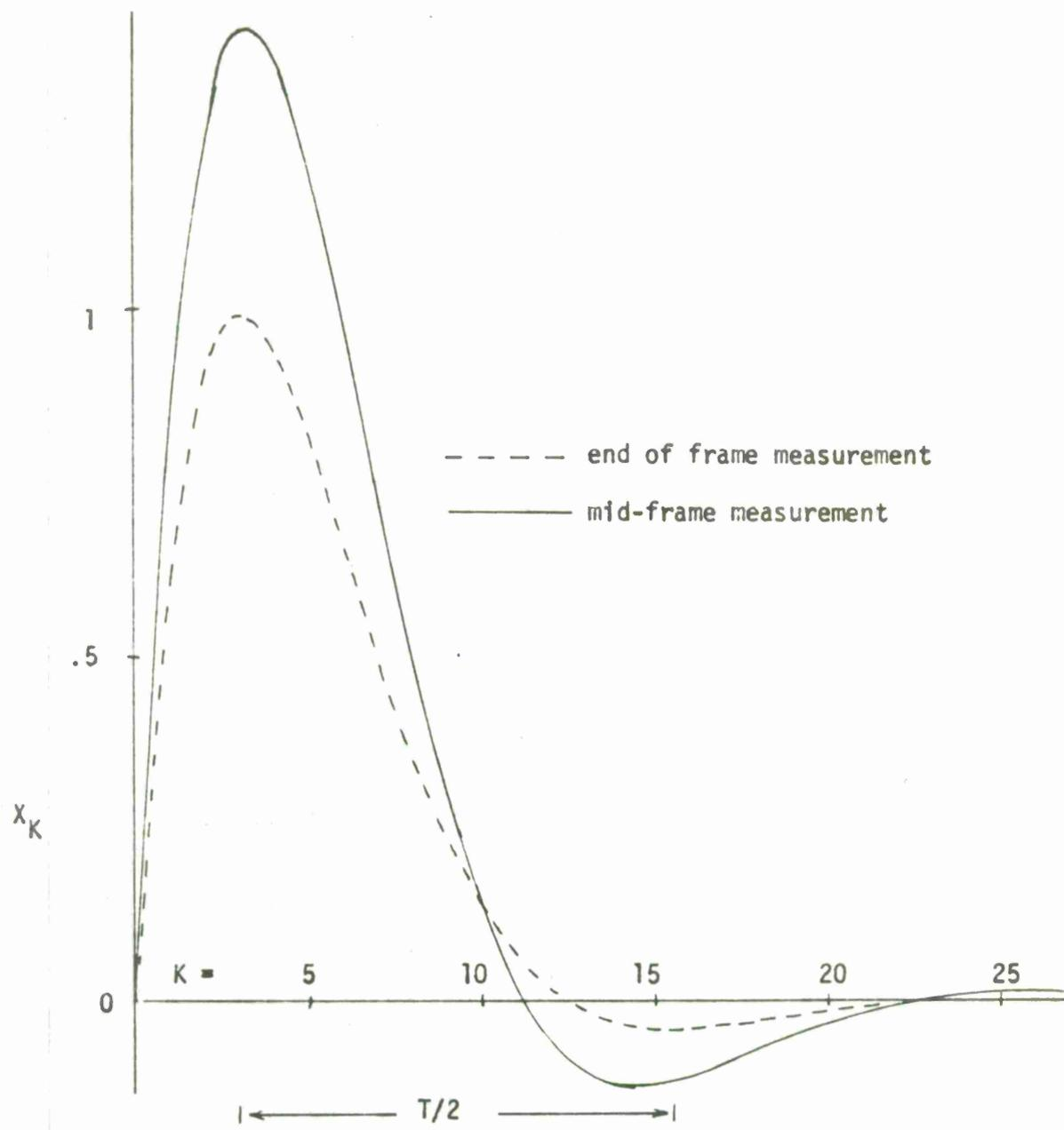
Figure 7. Unit Velocity Step Response
