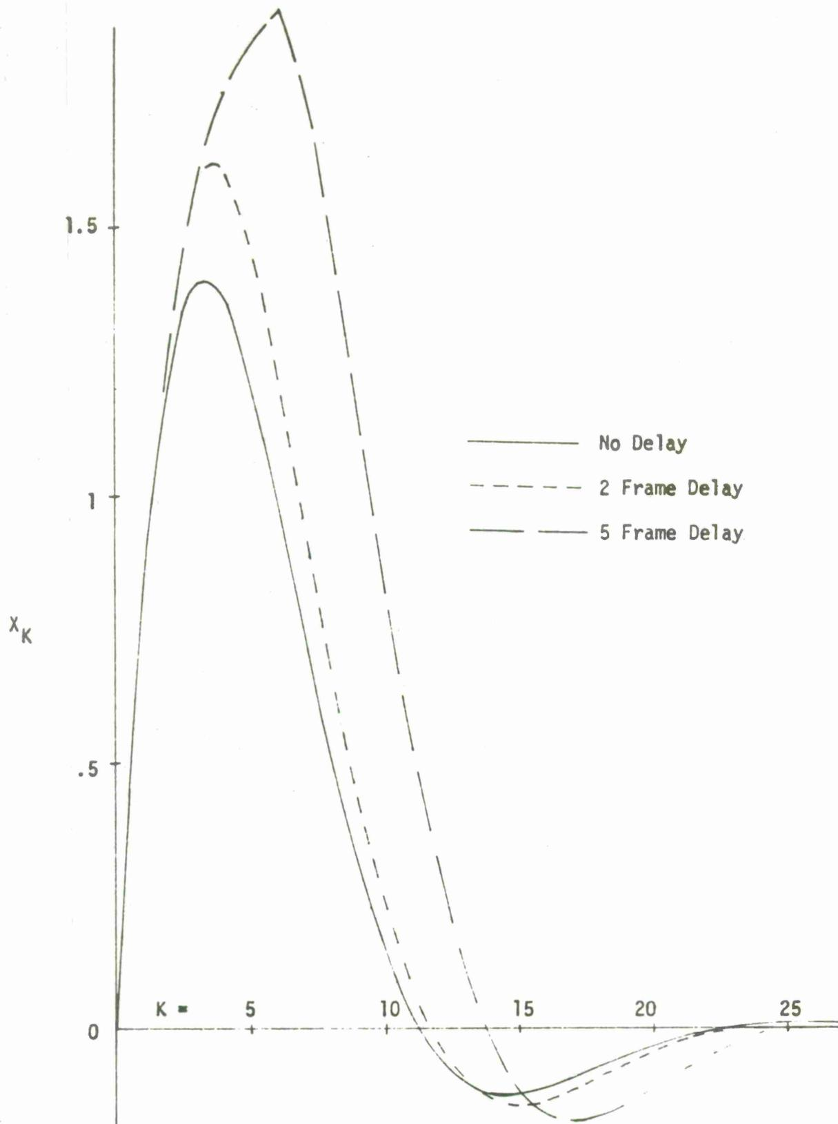
Figure 10. Effect of Delay in Rate Adjustment on Unit Velocity Step Response
