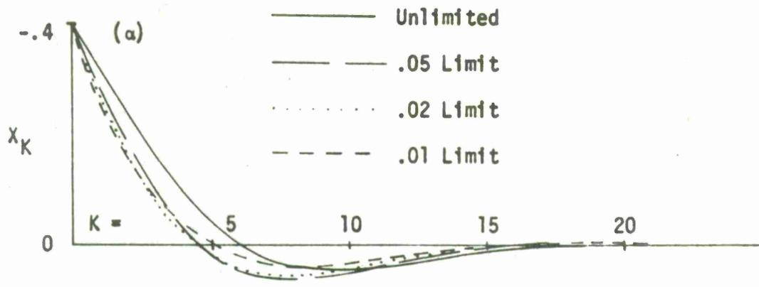
Figure 12a. Effect of Rate Limits on Unit Negative Impulse Response
