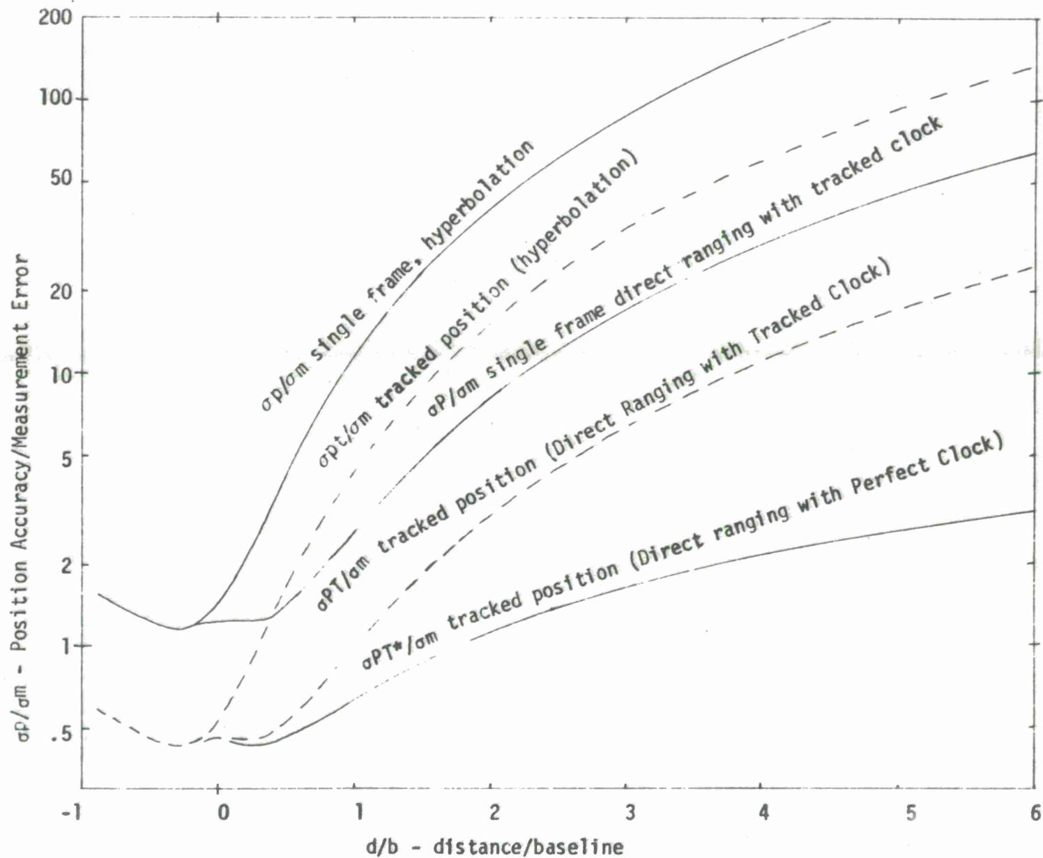
Figure 1 - Position Accuracy versus Distance from Baseline
