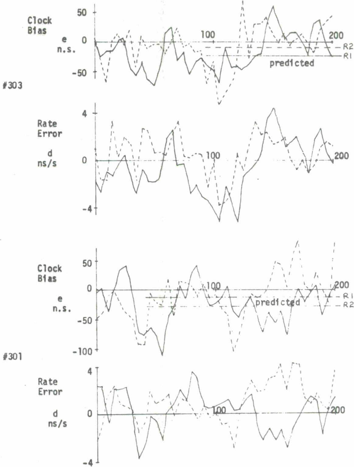
Figure 21. Reference--Steady State Clock Error for  $\alpha = 0.14$ ,  $\beta = .0182$
