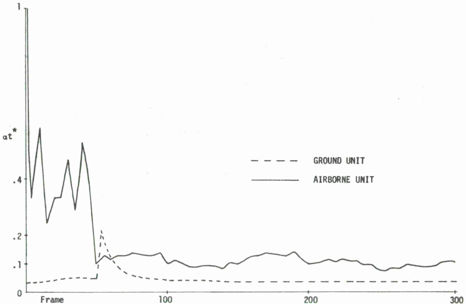
Figure 33. Effective Time Smoothing Constant,  $\alpha t^*$ , Run #306
