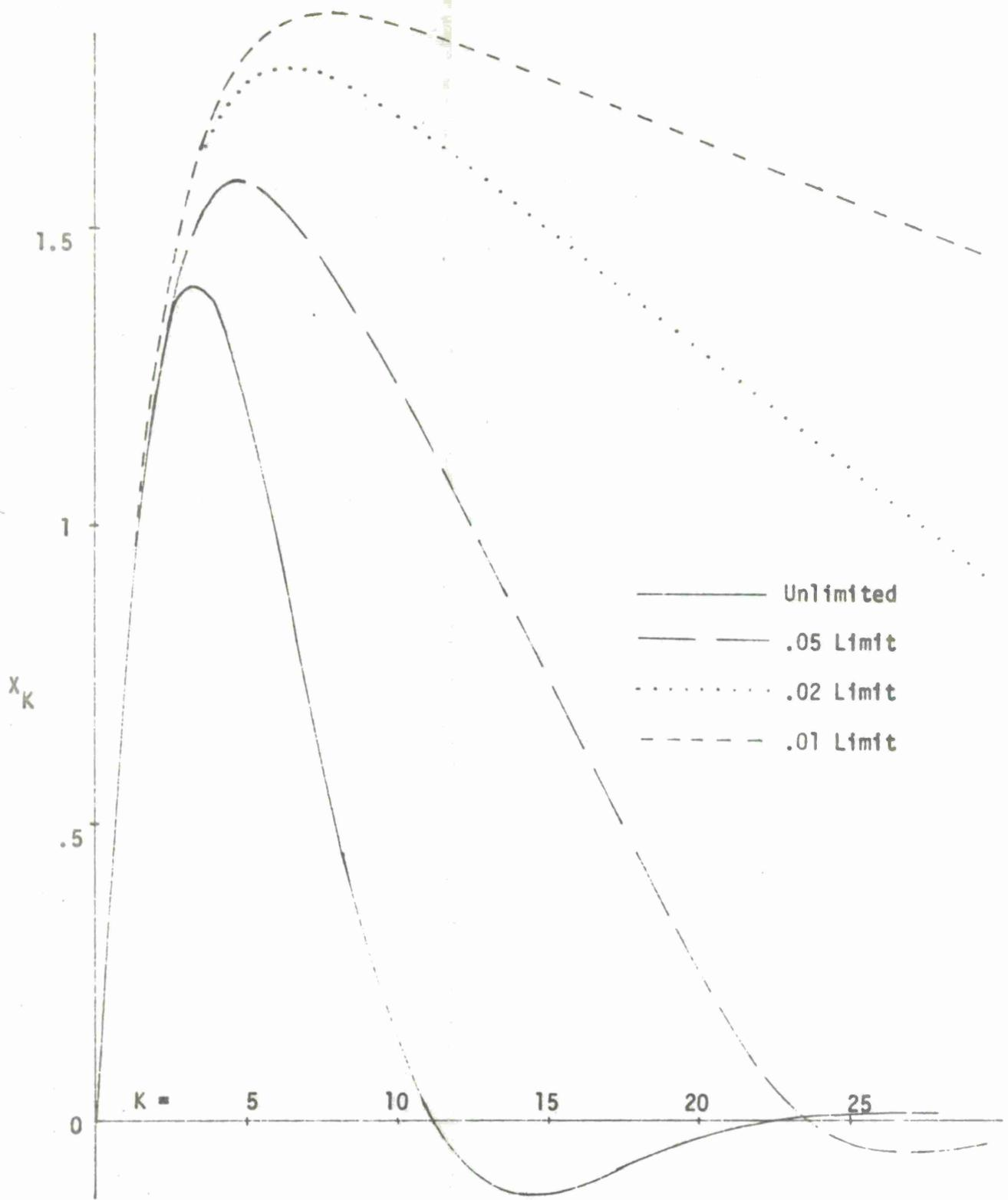
Figure 13. Effect of Rate Limits on Unit Velocity Step Response
