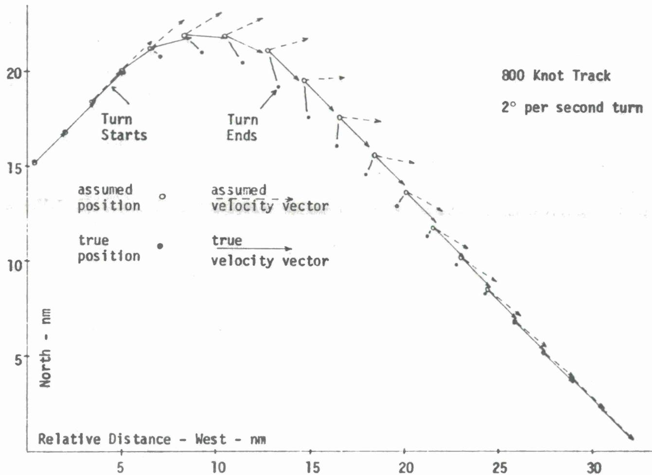
Figure 50. Example of Data Tracking Through 90° Turn
