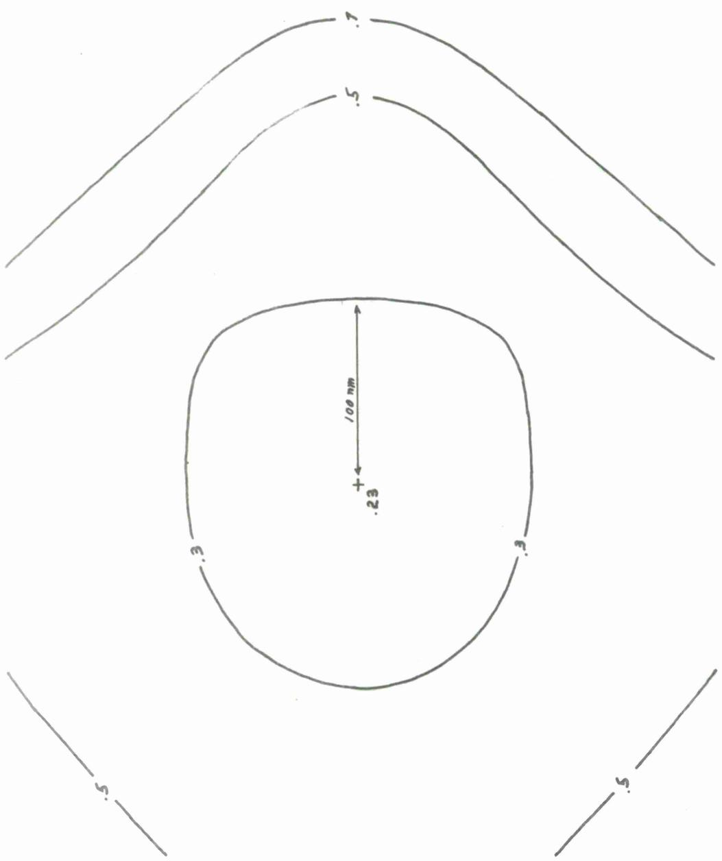
Figure 43. Contours of Tracked Position Accuracy (Direct Ranging),  $\sigma_{PT}/\text{cm}$ , Run #214 Area.
