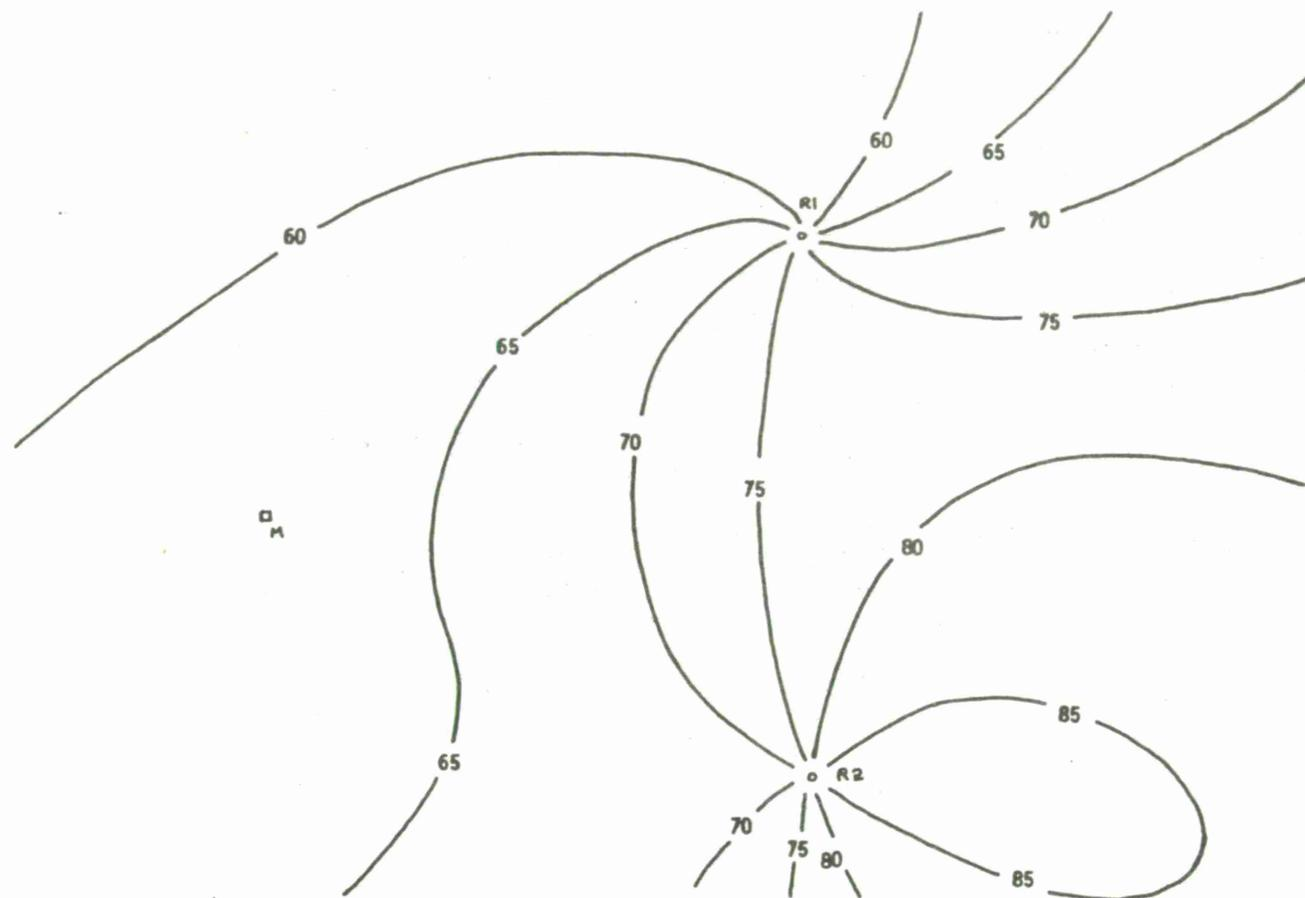
Figure 45. Clock Error Induced at Airborne Units in Triple Ground Cover due to Reference Bias of  $e_t = 100$  n.s. and  $e_p = 30$  feet. Expressed as  $e$  (nanoseconds) versus  $x, y$ . Run #214.
