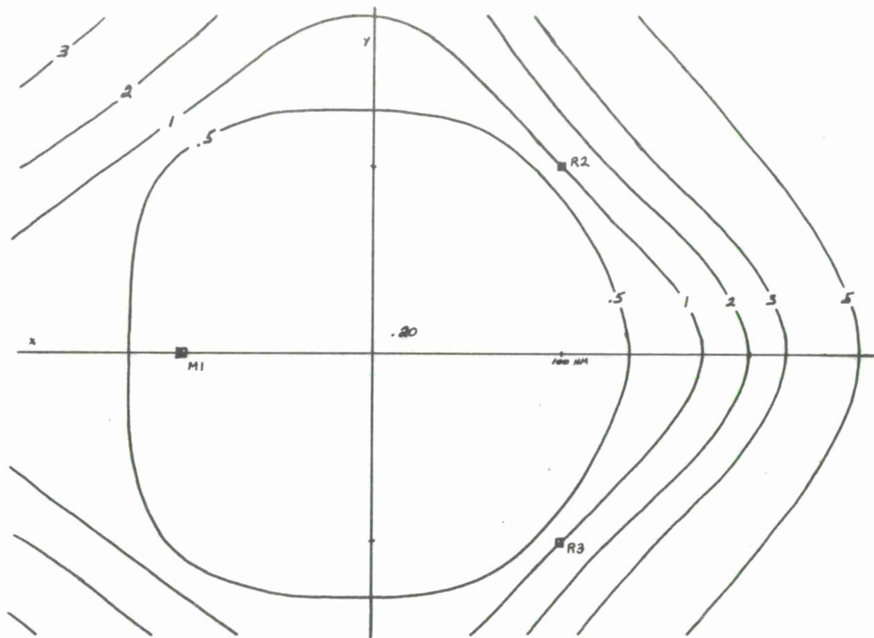
Figure 42. Geometric Dilution of Precision--Single Fix, Time. Five Reports per Frame from Three Imperfect References, plus Fifteen Airborne Sources.  $\sigma_t/\sigma_m$  versus  $x, y$ .
