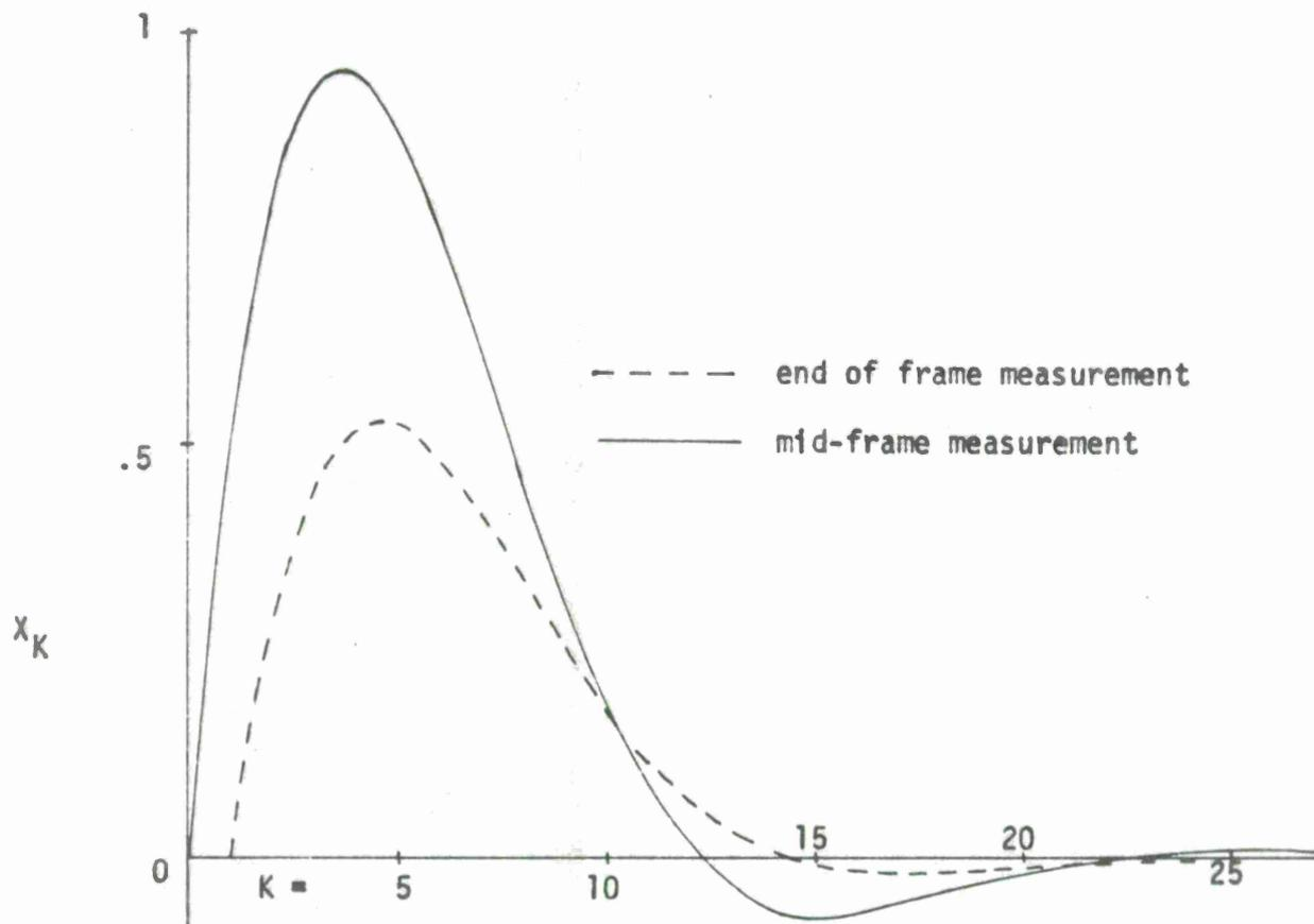
Figure 8. Modified  $\alpha - \beta$  Tracker, Unit Velocity Step Response
