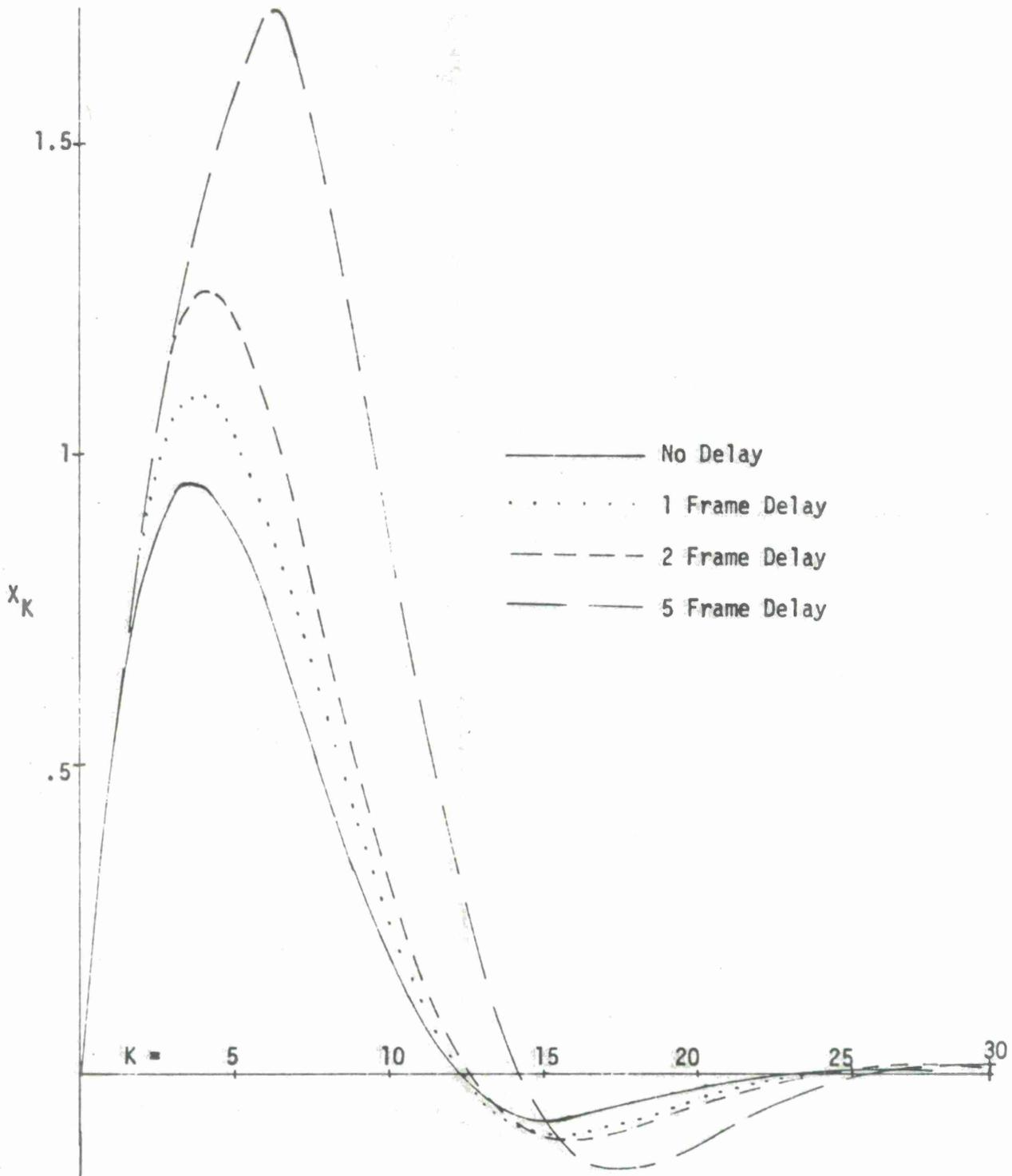
Figure 11. Effect of Delay in Rate Adjustment on Unit Velocity Step Response with Modified  $\alpha - \beta$  Tracker
