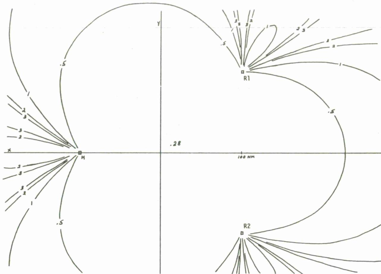
Figure 41. Direct Ranging, Theoretical Tracked Position Accuracy with Three Perfect References. Showing  $\sigma_{PT}/\sigma_M$  versus  $x, y$ .  $\alpha_t = .054, \alpha_p = .36$
