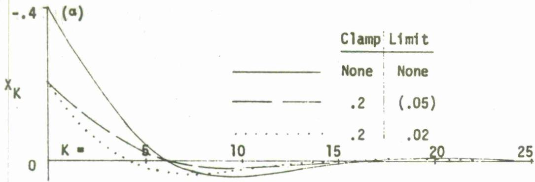
Figure 17.a. Solution Clamp and Rate Limit, Unit Negative Impulse Response
