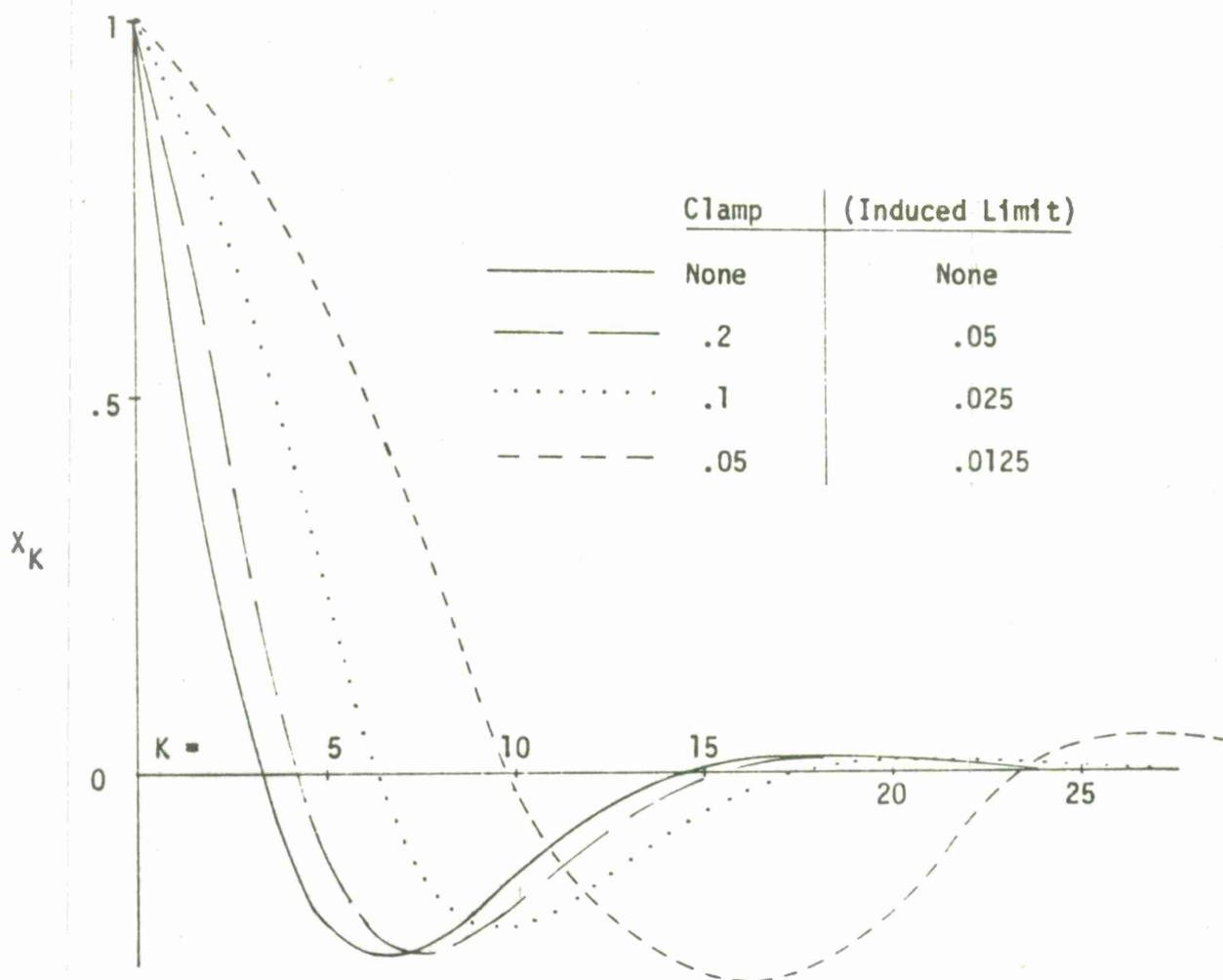
Figure 15b. Effect of Solution Clamp on Unit Position Step Response
