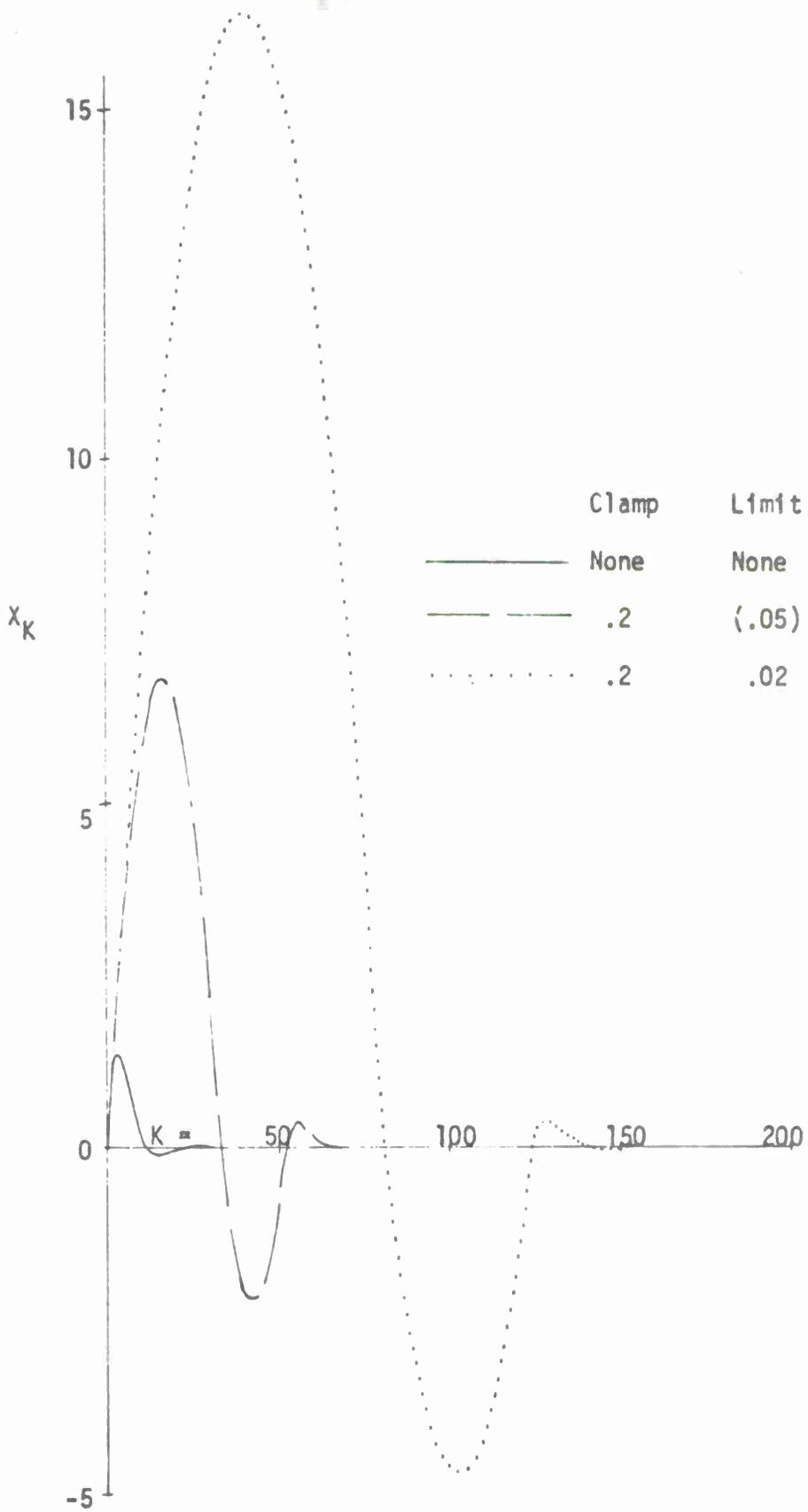
Figure 18. Solution Clamp and Rate Limit, Unit Velocity Step Response
