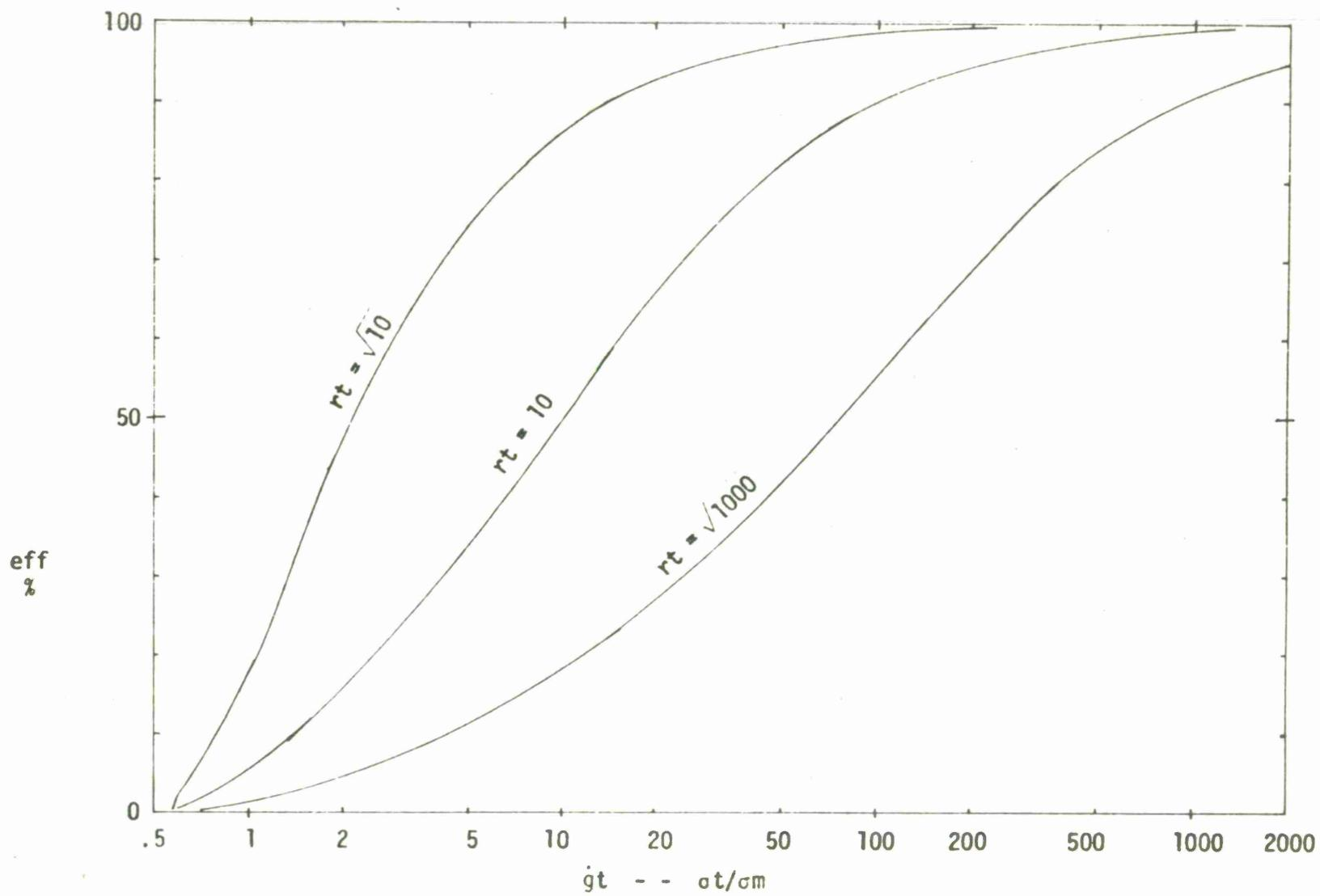
Figure 2. Efficiency Factor versus Geometric Dilution of Precision (Time)
