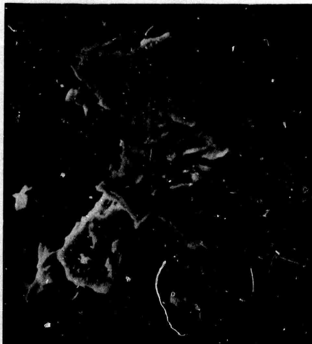
Figure 15. SEM Photomicrograph of Yttralox Oxalate Powder Calcined for 4 hrs at 800°C in Air X5000
