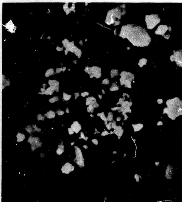
Figure 17. SEM Photomicrograph of Ball-Milled Yttralox Powder X10,000
